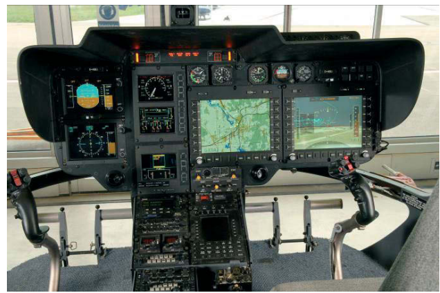
Figure 7: Special instrument panel of EC145 test bed.
