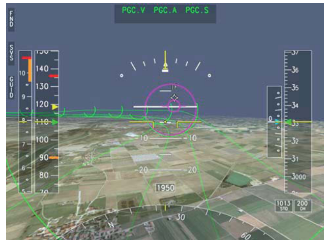
Figure 9: Helicopter specific tunnel symbology.
