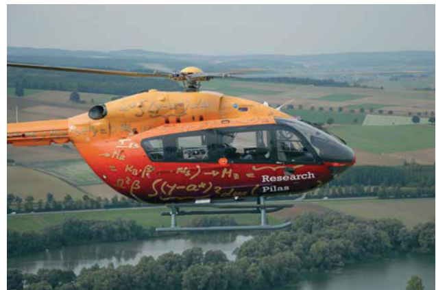
Figure 2: PILAS flying research test bed – an EC145
