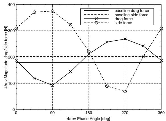
Figure 5: 4/rev drag and side force at rotor hub vs. IBC phase angle for single harmonic 4/rev collective control with amplitude 0.2 deg,  $\mu = 0.26$
