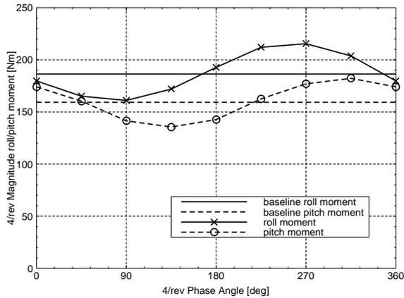
Figure 6: 4/rev roll and pitch moment at rotor hub vs. IBC phase angle for single harmonic 4/rev collective control with amplitude 0.2 deg,  $\mu = 0.26$
