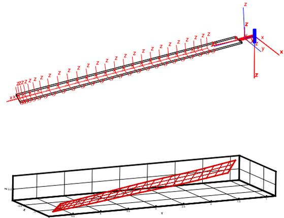
Figure 4: Aerodynamic Discretization of the blade
