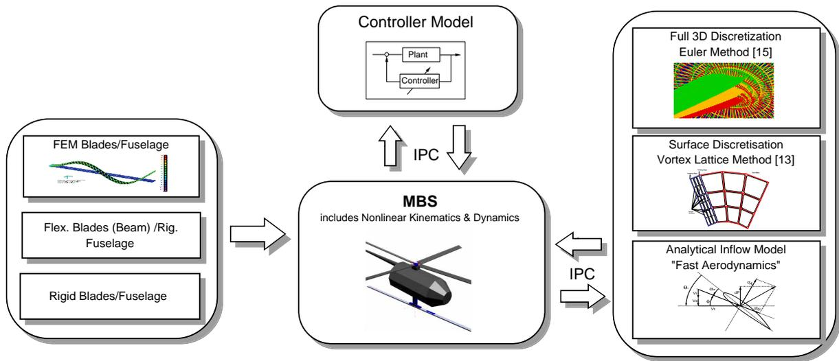
Figure 2: Modular Modeling and IPC Simulation Interfaces
