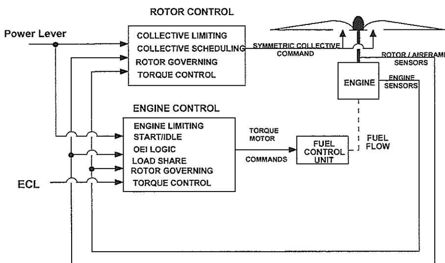
**Fig. 12. Torque command regulating system control laws.**
