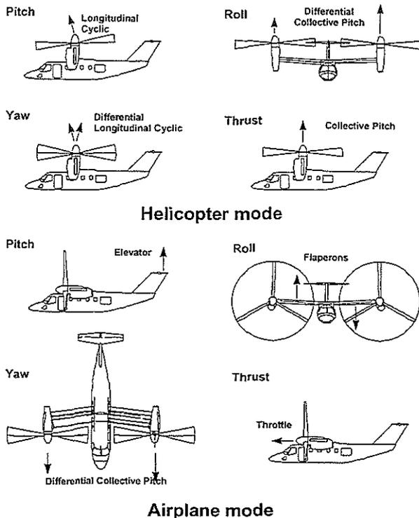
Fig. 2. BA 609 primary control mechanisms.
