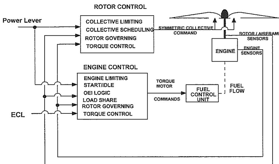
**Fig. 12. Torque command regulating system control laws.**
