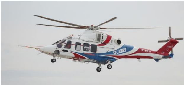
Figure 1 T625 Gökbey Helicopter with air data boom
