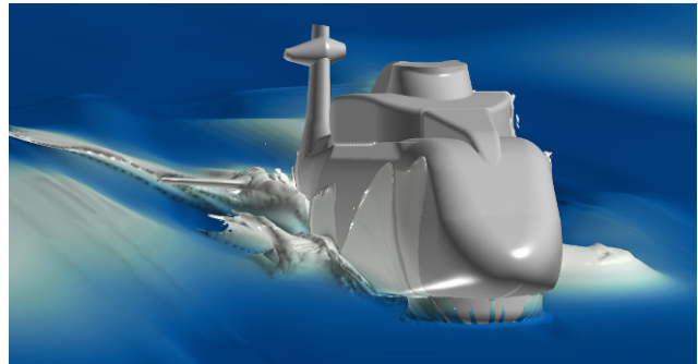
Figure 5 – CFD simulation of AW101 for calibration of hydrodynamic pressures
