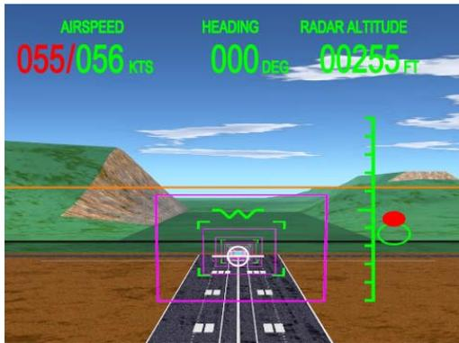
**Fig. 4 Head up display used for PAV manual landing**
