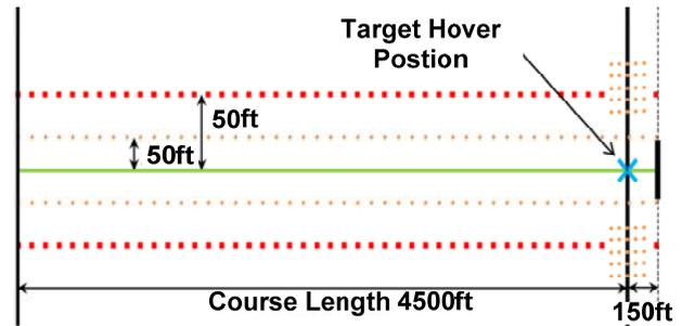
**Fig. 2 General plan-view arrangement for decelerating descent manoeuvre**
