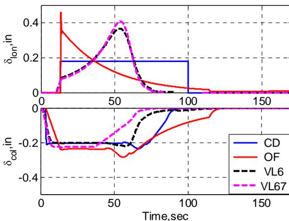
**Fig. 7 Pilot model inputs for each of the designed profiles**
