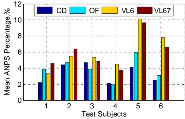
**Fig. 12 Mean attack number per second of longitudinal control input (manual landing)**
