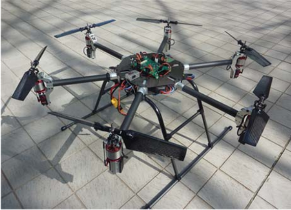
Figure 1: A variable pitch-angle controlled multicopter prototype
