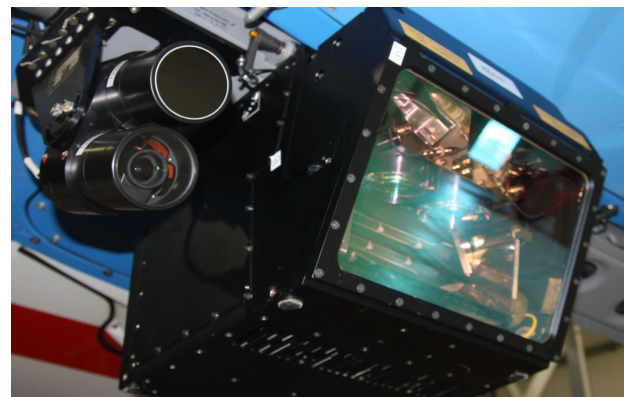
Figure 2: SferiSense® 300 (right) and TV and IR cameras (both used for recording only)
