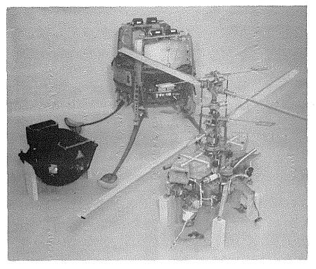
FIG. 8 WIDEYE MODULAR CONSTRUCTION
