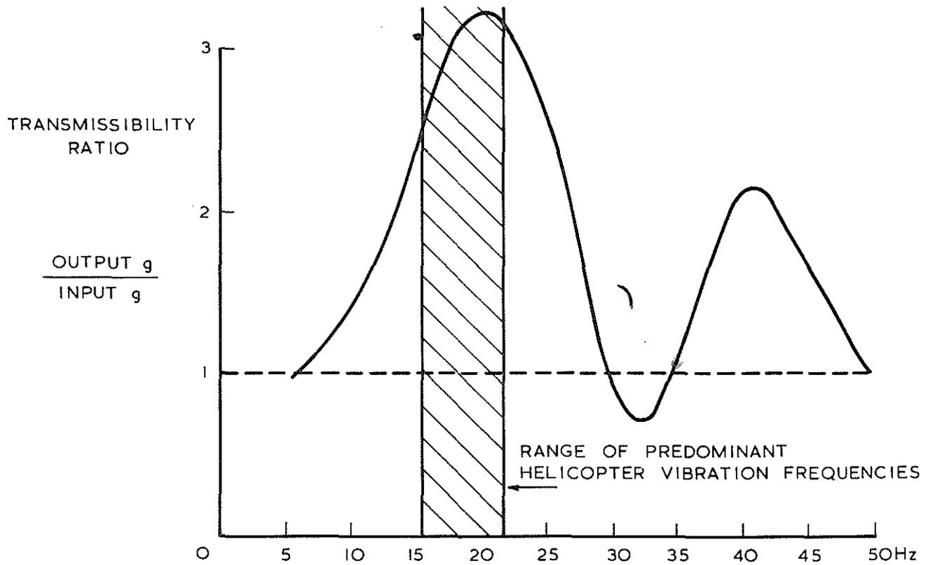
Fig 5 Transmission of vertical vibration to equipment through anti-vibration mounts
