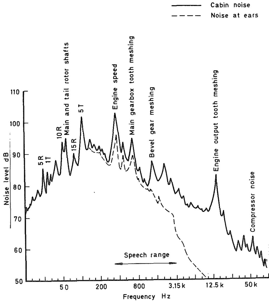
Fig 6 Typical gas turbine powered helicopter noise spectrum
