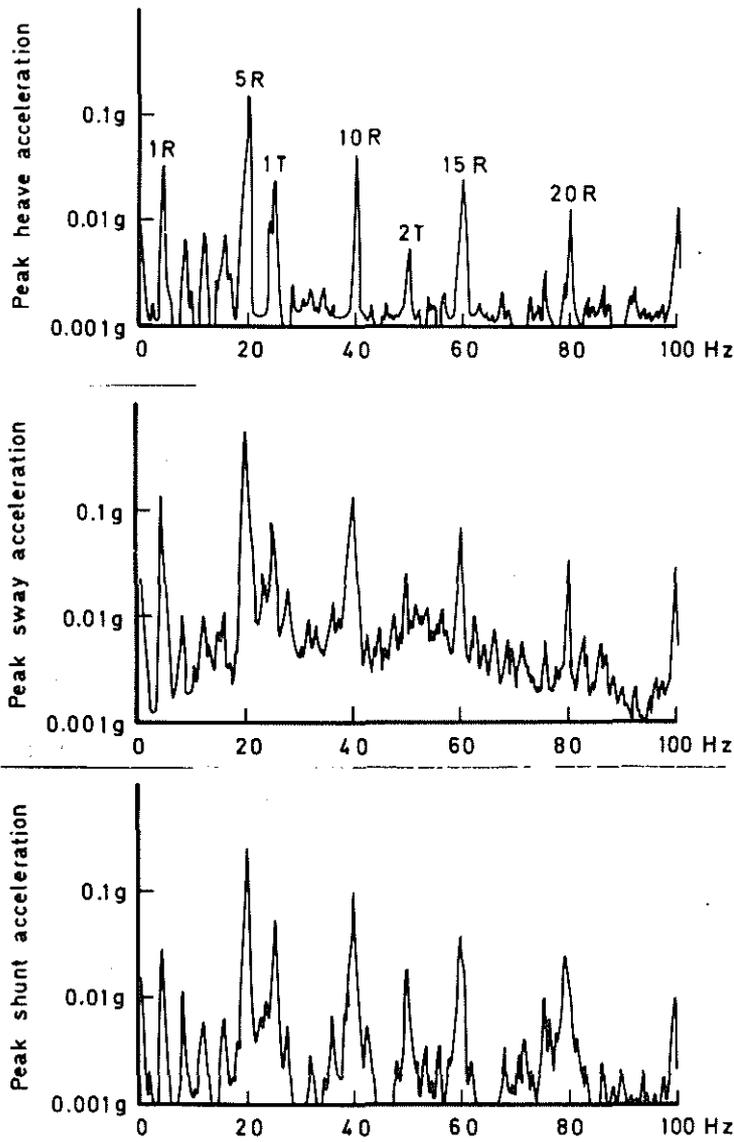
Fig 3 Vibration frequency spectra at pilot's seat position in a typical 5 bladed medium sized helicopter
