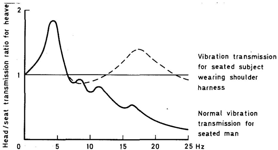
Fig 4 Heave vibration transmission from seat to head for a seated man, with and without shoulder harness
