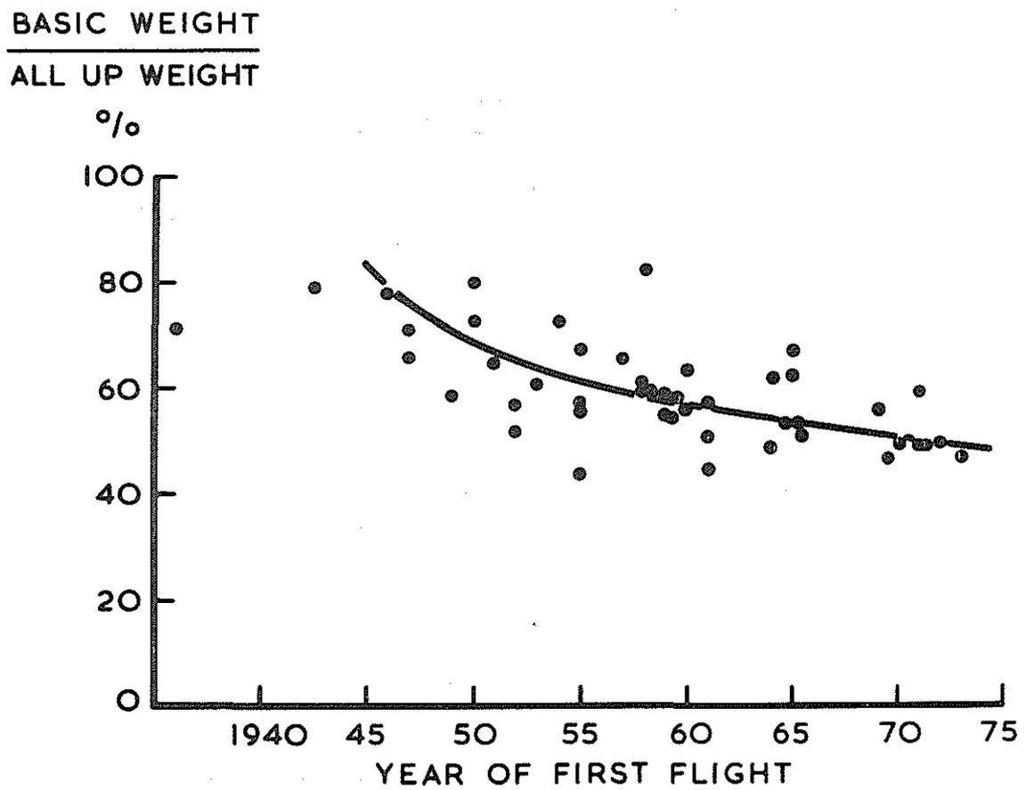
Fig 2 Improvement of lifting ability with time
