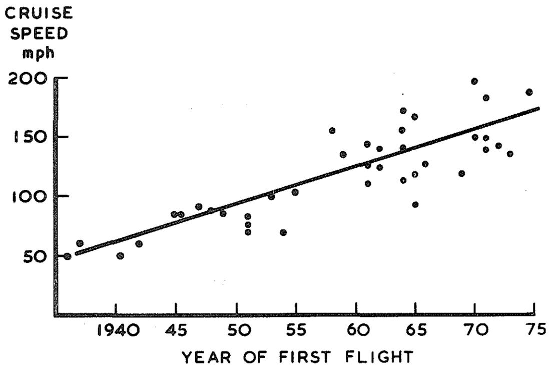
Fig 1 Speed increase with time
