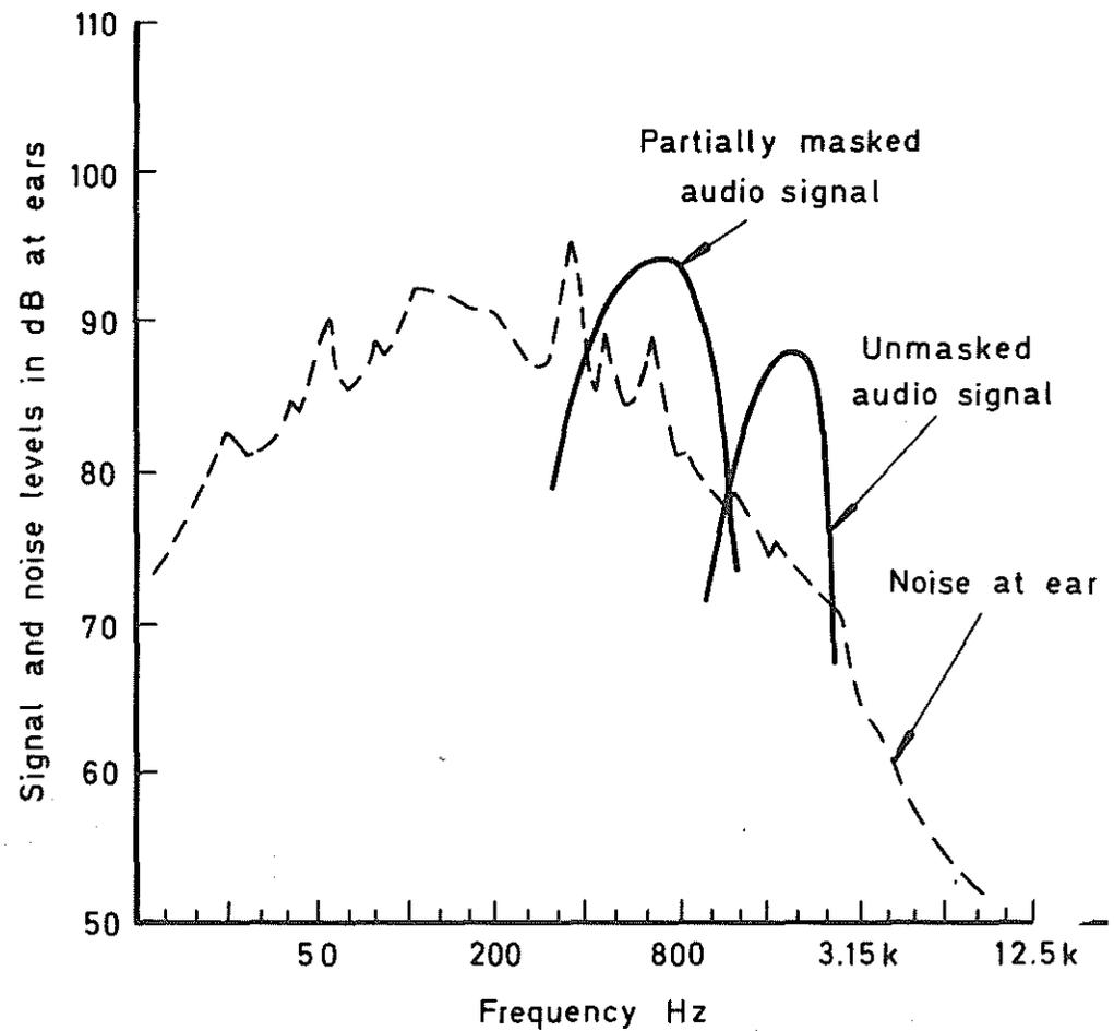
Fig 7 Noise and signals at ears of crew
