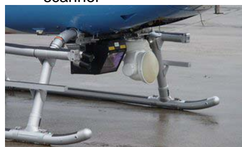
Figure 1: ALLFlight sensors mounted between the landing skid
