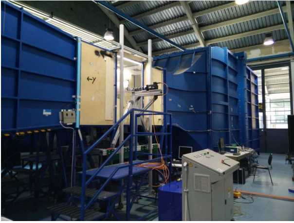
Figure 1: The oscillating airfoil test rig installed at the S. De Ponte wind tunnel of Politecnico di Milano.
