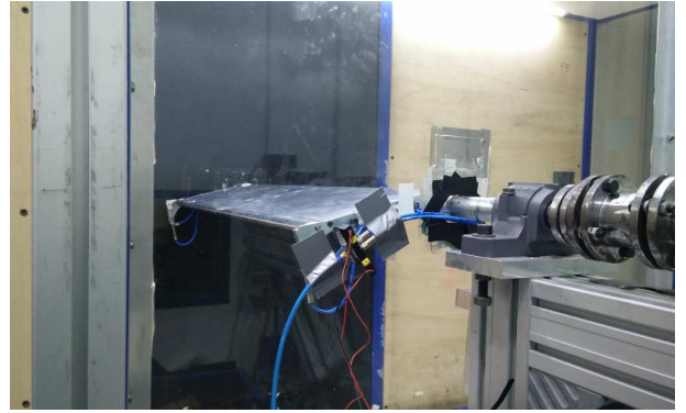
Figure 4: The NACA 23012 airfoil model equipped with the L-shaped tab in the wind tunnel test section.
