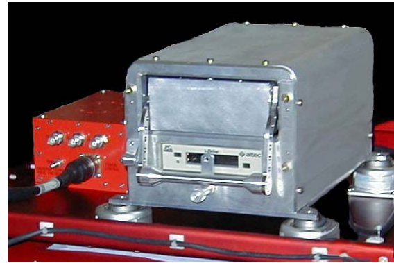
Fig. 6: Data Storage Device
