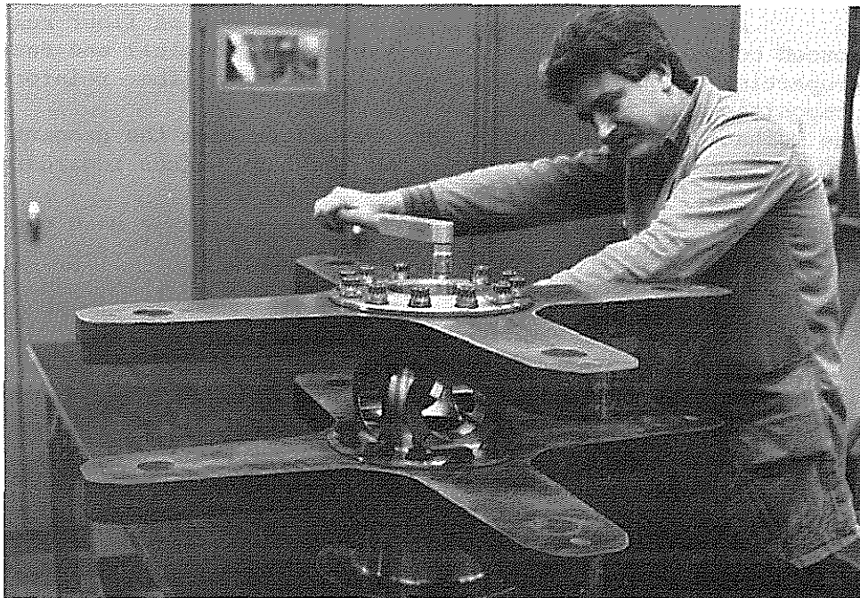
Figure 2: Rotor hub with plates out of GFC
