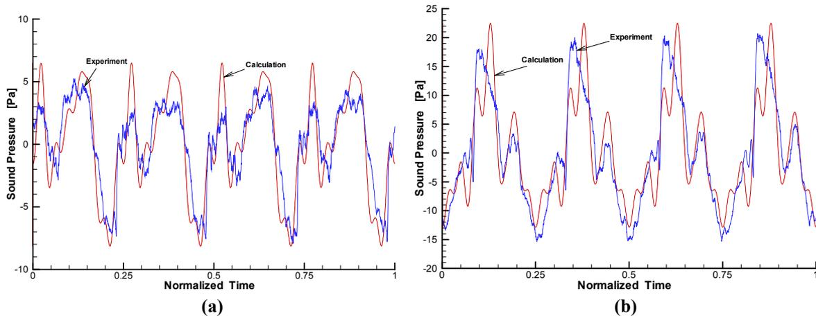
Figure 7: TC067: comparison of acoustic experimental and simulated signature at microphone 1 (a) and 2 (b)
