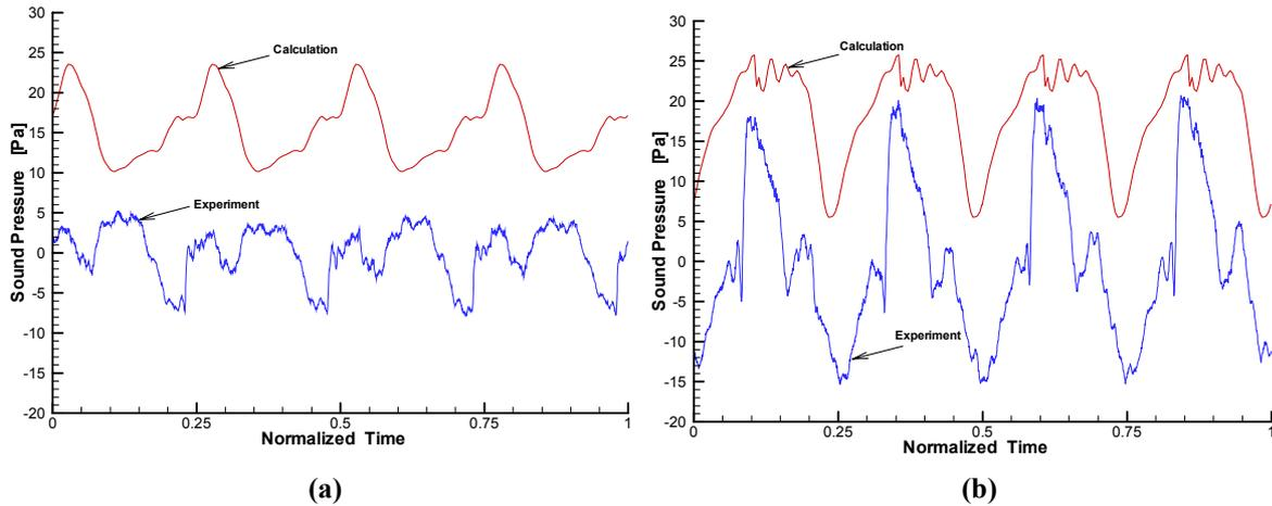
**Figure 12: TC067: comparison of acoustic experimental and simulated signature at microphone 1 (a) and 2 (b)**
