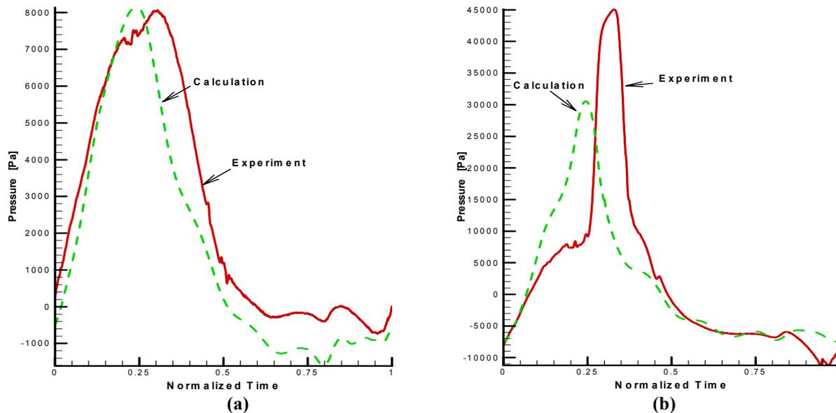
**Figure 14: Comparison of experimental and simulated blade pressure time histories on probes located near trailing edge at middle spanwise (a) and near leading edge in the tip region (b)**
