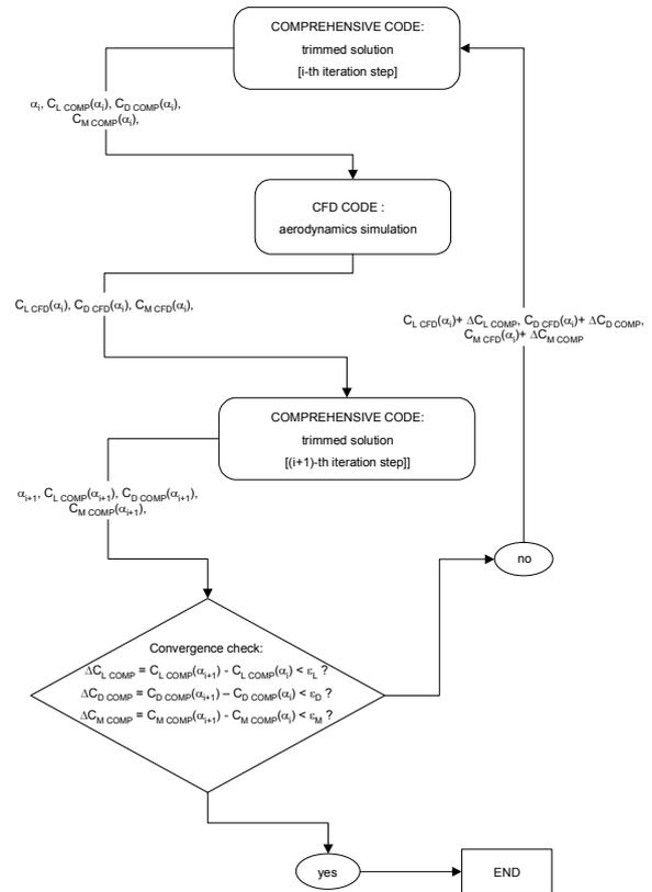
**Figure 3: Aeroelasticity-Aerodynamics coupling technique**
