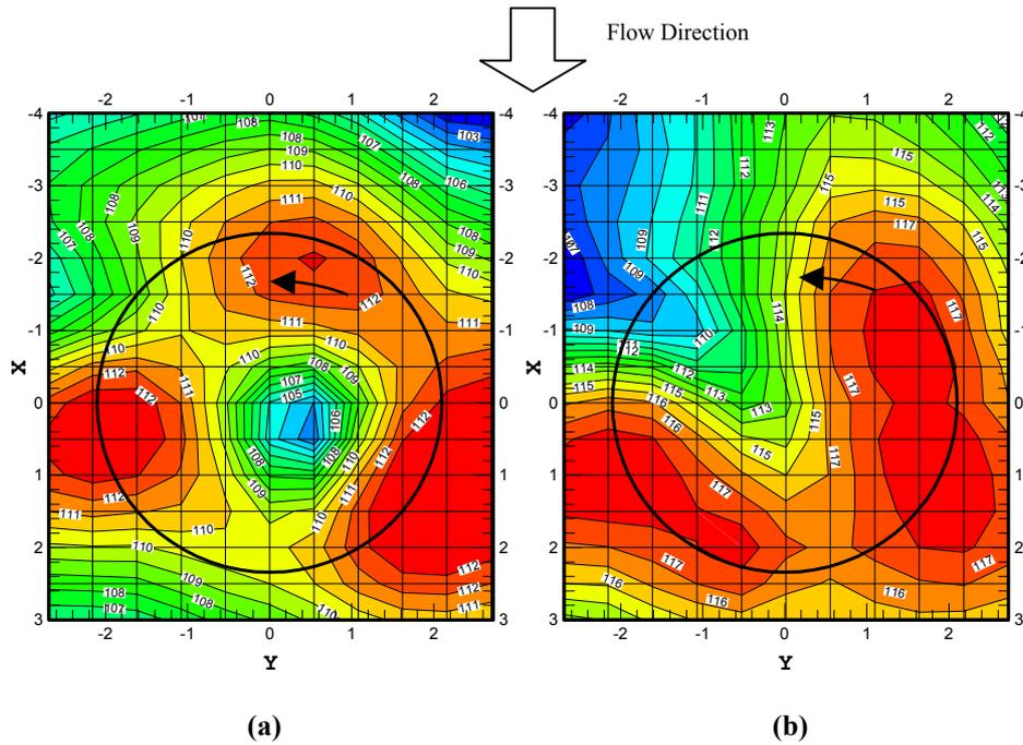
Figure 10:TC067: comparison between simulated (a) and experimental (b) noise footprint
