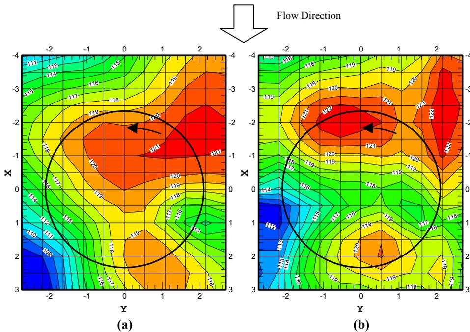
Figure 6: TC152: comparison between simulated (a) and experimental (b) noise footprint
