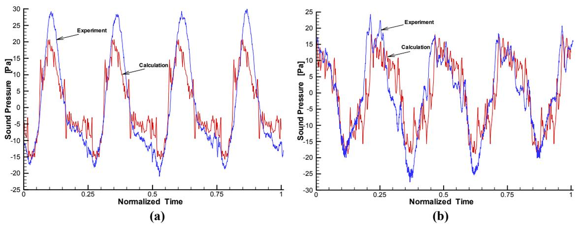
Figure 8: TC152: comparison of acoustic experimental and simulated signature at microphone 1 (a) and 2 (b)
