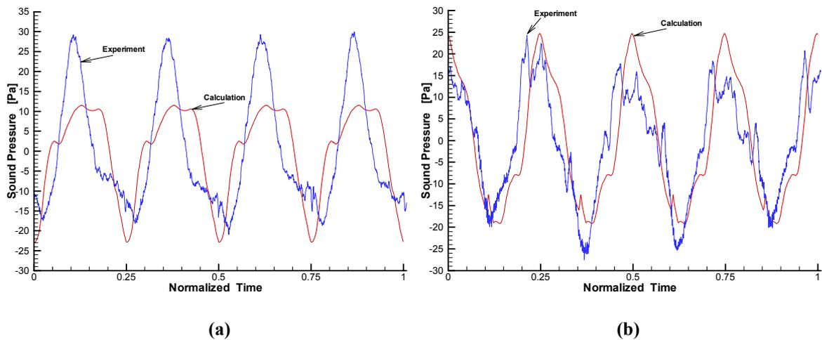
**Figure 13: TC152: comparison of acoustic experimental and simulated signature at microphone 1 (a) and 2 (b)**
