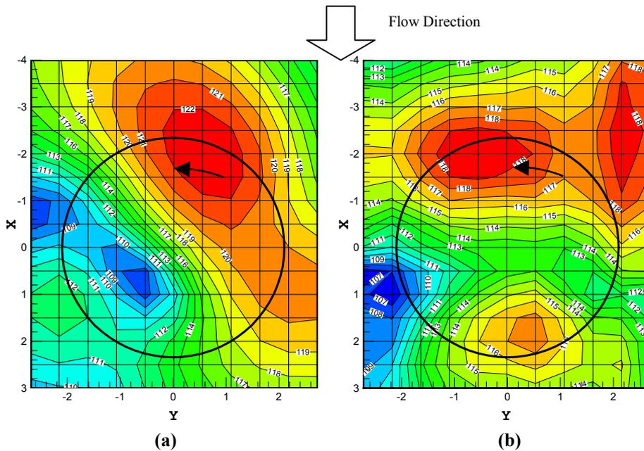
Figure 11:TC152: comparison between simulated(a) and experimental (b) noise footprint
