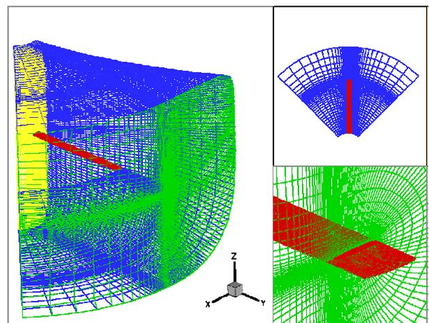
Figure 9: Computational grid over 7A blade for aerodynamic calculation
