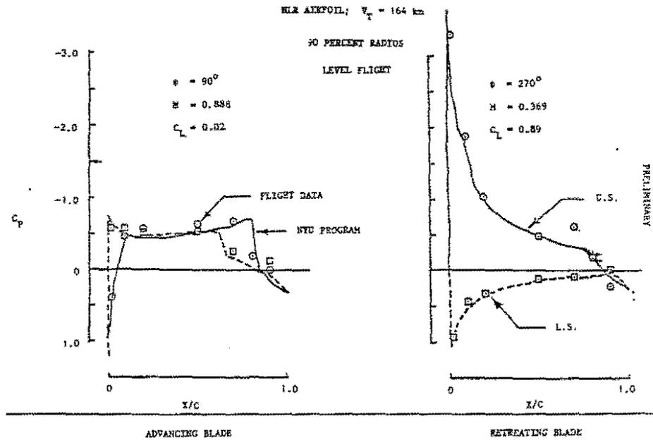
Fig 5 Measured and calculated chordwise pressure distributions — Langley/AH-1G
