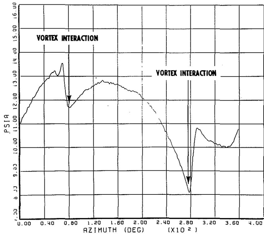
Fig 16 Blade leading edge absolute pressure distribution indication vortex interaction locations
