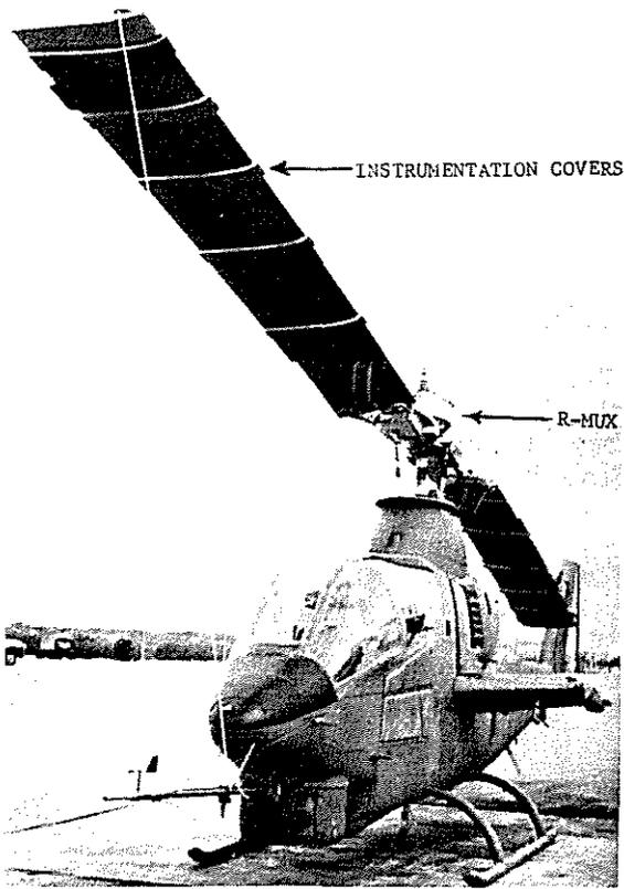
Fig 1 Army AH-1G with instrumented rotor
