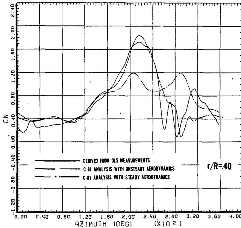
Fig 14 Normal force coefficient distribution comparing the effects of predicted unsteady aerodynamic representation at 0.31 advance ratio
