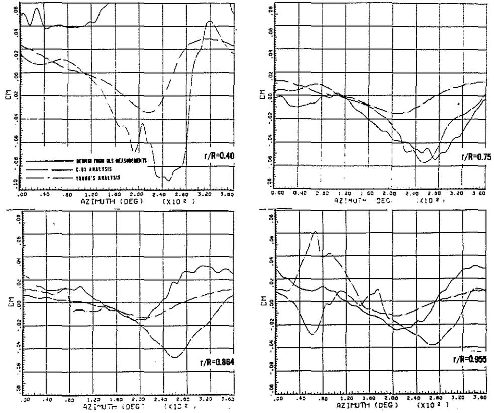
Fig 15 Quarter chord pitching moment coefficient distributions for various radial stations on the AH1G rotor at 0.31 advance ratio
