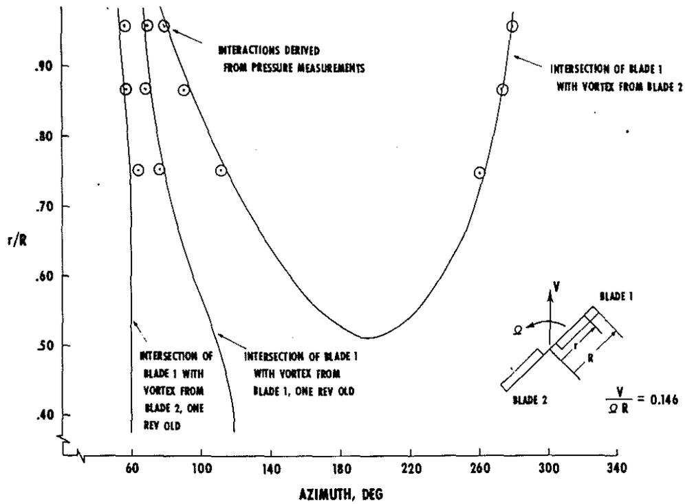
Fig 17 Comparison of vortex interactions derived from cycloid equations and measured data
