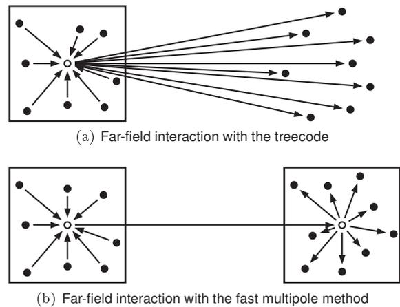
Figure 20: Differences between the treecode (a) and the fast multipole method (b) in calculating far-field influences.
