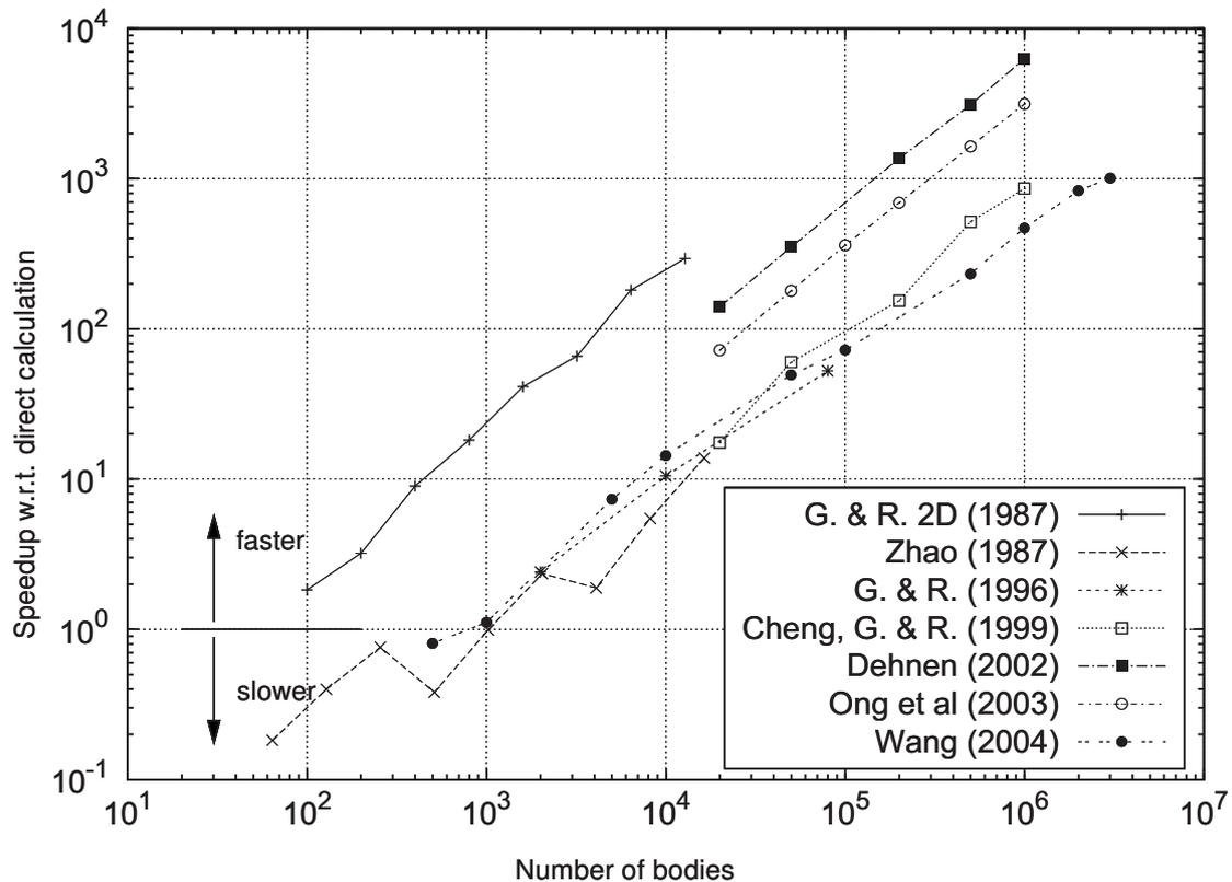
Figure 21: Comparison of speed improvements of various implementations of the Fast Multipole Method compared with the direct calculation. All implementations except for the first are in 3D, they are: <sup>[35;42;59;60;96;146;157]</sup>
