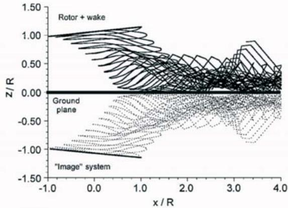
Figure 12: Example of predicted wake geometry using method of images to simulate ground effect, four-bladed rotor,  $C_T = 0.008$ , forward shaft tilt  $\alpha_s = 10$  deg. From Leishman, Bhagwat and Bagai<sup>[89]</sup>
