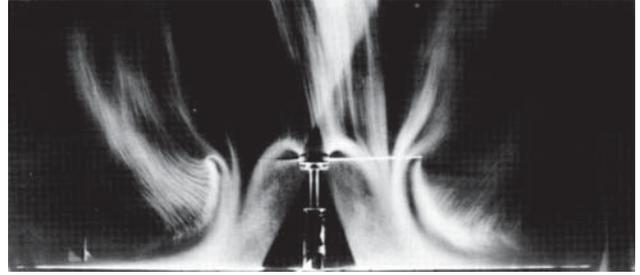
Figure 16: Flow near a rotor operating 1 radius above the ground visualised using balsa dust, reproduced from Taylor<sup>[138]</sup>
