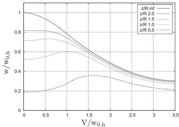
Figure 17: Induced velocity at the centre of the rotor in forward flight near the ground, x-axis: rotor forward velocity, y-axis: induced velocity at rotor centre; both nondimensionalised by hover induced velocity OGE<sup>[69]</sup>
