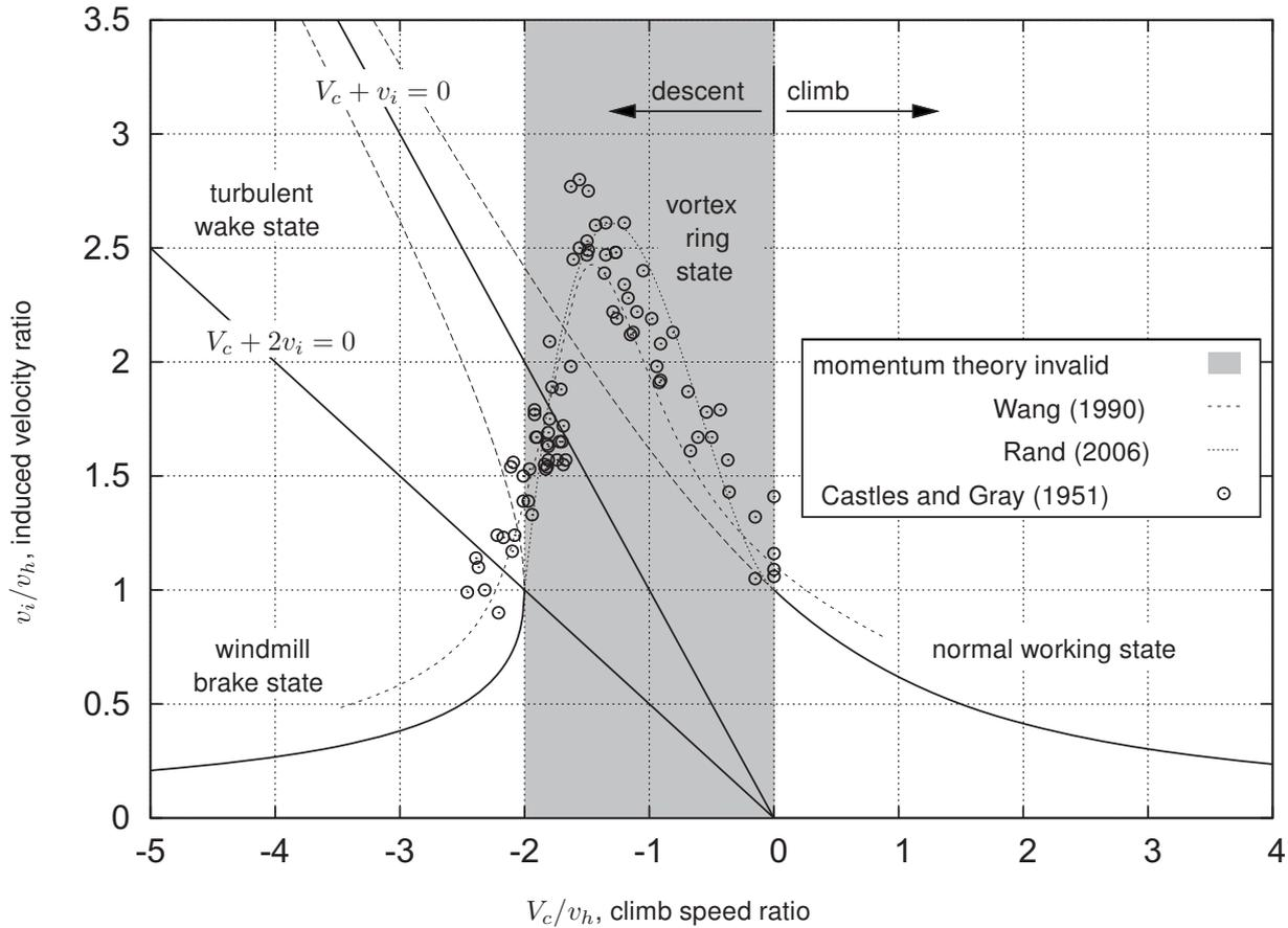
Figure 2: Rotor induced velocity as a function of climb speed ratio, showing the different branches of the analytical model. The experimental data was extracted from a NACA report by Castles and Gray<sup>[143]</sup>
