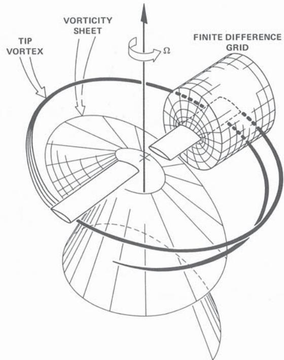
Figure 14: A finite-difference model embedded in a global hover flow, showing the disparity between a typical blade-oriented grid and the total hovering flow field<sup>[27]</sup>.
