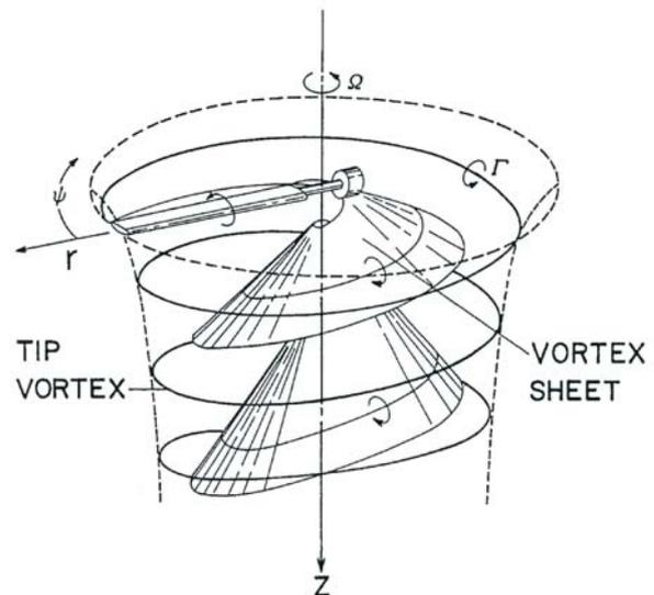
Figure 5: Geometry of the wake of a single-bladed hovering rotor as determined from flow visualisation studies, from Gray<sup>[57]</sup>.
