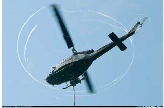
Figure 8: Tip vortex made visible through condensation of water vapour inside the vortex core of a Bell 214B-1 helicopter. Image source <http://www.airliners.net>, © Bill Campbell, used with permission.
