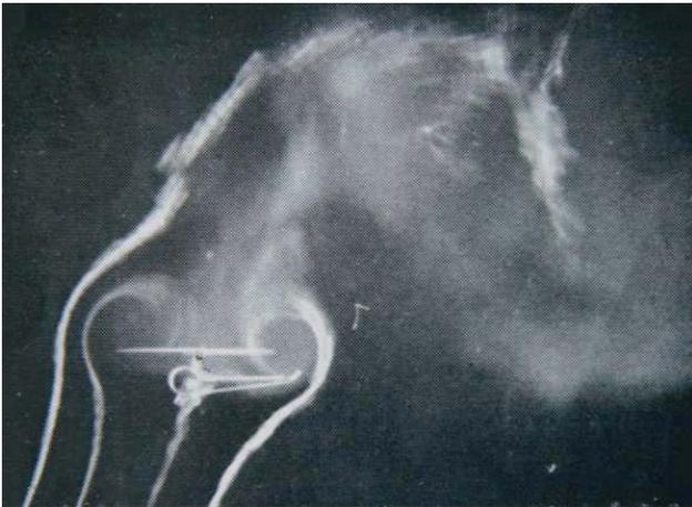
Figure 3: Smoke visualisation of helicopter rotor in vortex ring state<sup>[46]</sup>
