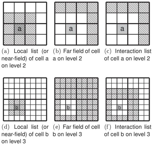
Figure 19: Near field, far field and interaction list for cells on level two and three in a quadtree.
