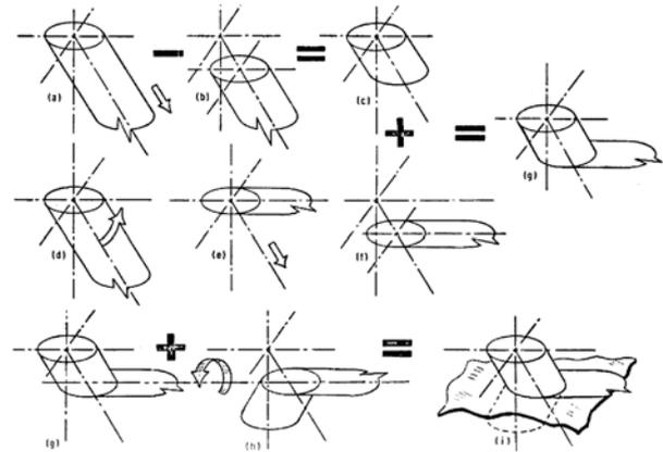
Figure 18: Superpositions of the wake and its associated flow field used to obtain the wake and flow field in ground effect<sup>[70]</sup>
