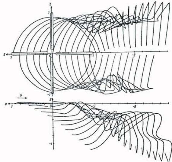
Figure 10: Rotor tip vortex geometry in low speed forward flight at low advance ratio ( $\mu = 0.1$ ) and tip path plane angle of attack  $\alpha = 11^\circ$ .<sup>[139]</sup>
