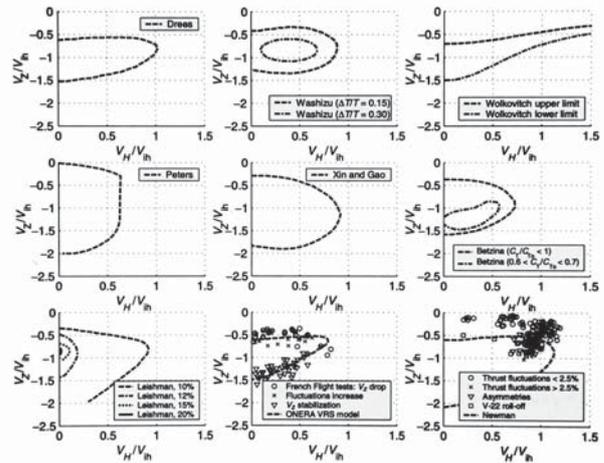
Figure 4: Vortex Ring State boundaries as determined by various studies<sup>[14]</sup>.
