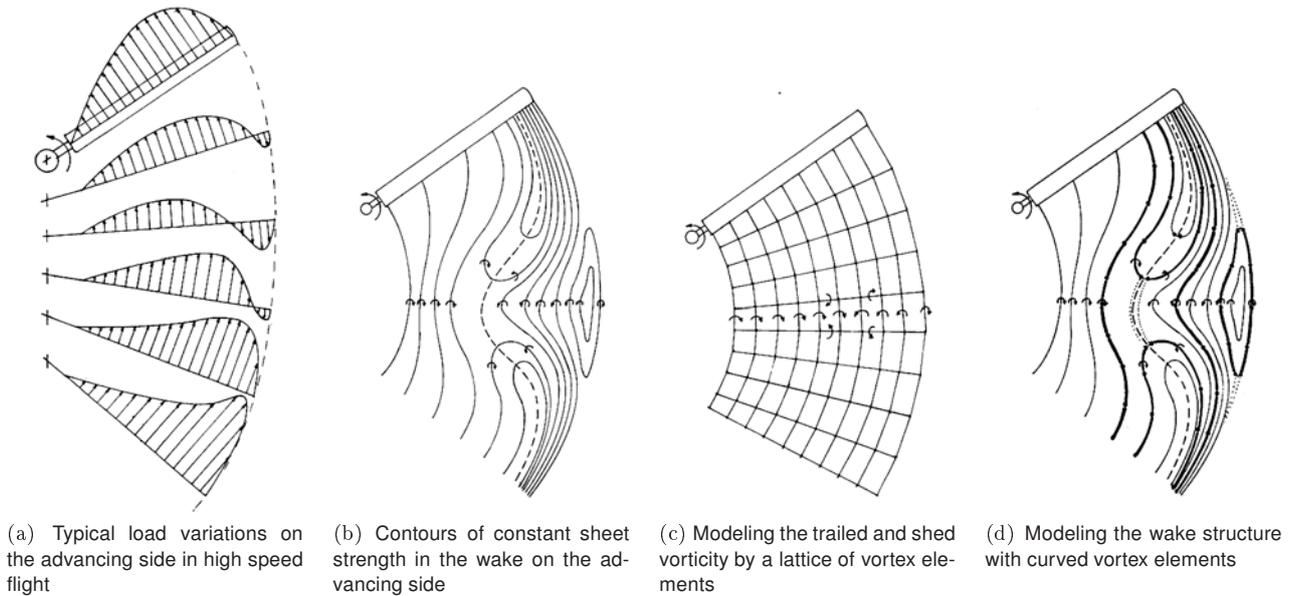
Figure 11: Modeling the structure of the wake using lattice and constant vorticity contour elements<sup>[107]</sup>.
