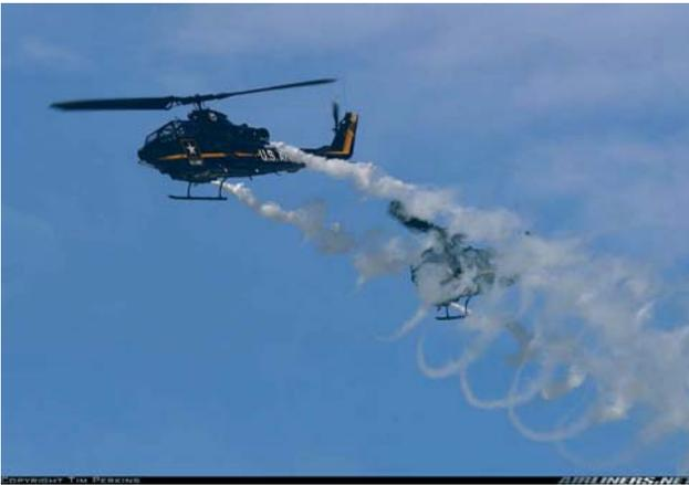
Figure 7: Near-field tip vortex wake made visible with smoke dispersed by a AH-1F Cobra at the Alliance 2007 Airshow in Ft. Worth. Image source <http://www.airliners.net>, © Tim Perkins, used with permission.
