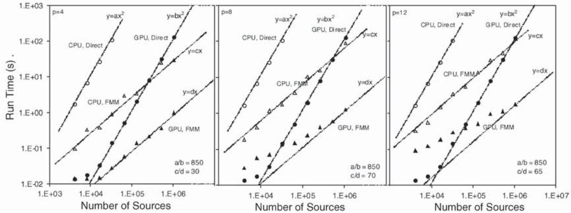
Figure 22: FMM wall clock time (in seconds) for serial CPU (one core of 2.67 GHz Intel Core 2 extrem QX is employed) and for GPU (NVIDIA GeForce 8800 GTX) for different truncation numbers  $p$  (potential+gradient). Also direct summation timing is displayed for both architectures. No SSE optimizations for the CPU were used<sup>[61]</sup>.
