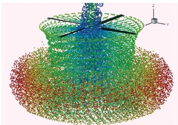
Figure 13: Rotor vortex particle wake visualisation of a rotor in hover after 8 revolutions using GENUPV<sup>[97]</sup>.
