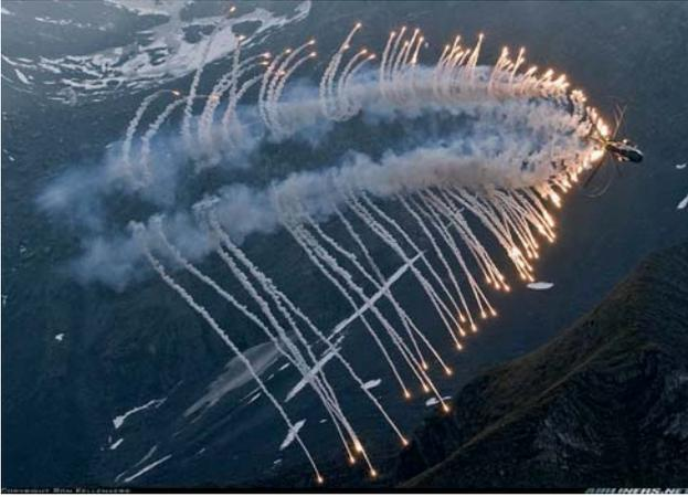
Figure 6: Far-field rotor wake made visible with the smoke of flares dispersed by a Eurocopter Cougar of the Swiss Armed Forces on October 10, 2007. Image source <http://www.airliners.net>, © Ron Kelleners.
