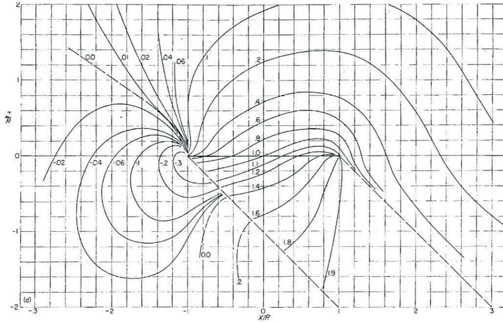
Figure 9: Induced flow near a rotor in forward flight with a wake skew angle of  $45^\circ$ , from Castles and de Leeuw<sup>[29]</sup>.
