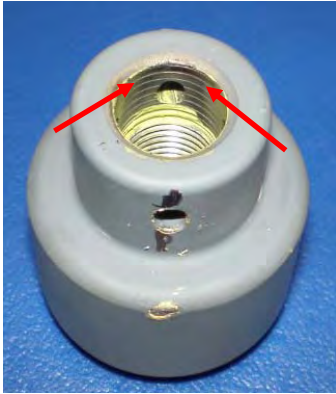
Figure 12. Markings on the inner side of the propeller moment weight
