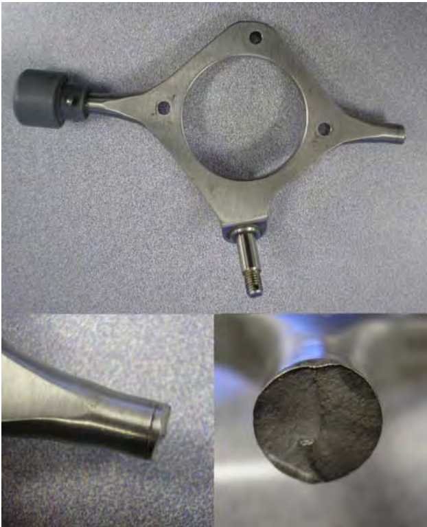
Figure 10. Rupture of the attachment arm of the propeller moment weight
