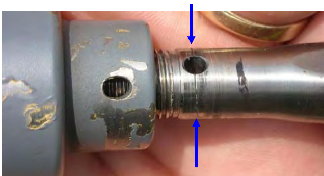
Figure 17. Broken control lever arm in the area of the cotter pin borehole
