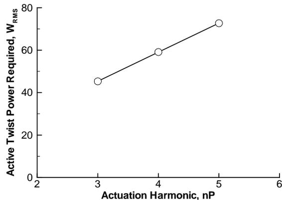
Figure 20. Rotor actuation power required.
