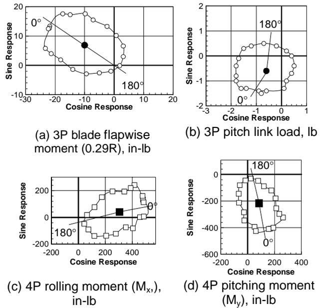
Figure 11. Rotating- to fixed-system loads comparison for  $\mu = 0.140$ ,  $C_L = 0.0066$ ,  $\alpha_s = -1.0^\circ$ , and 3P, 1000 V IBC actuation.
