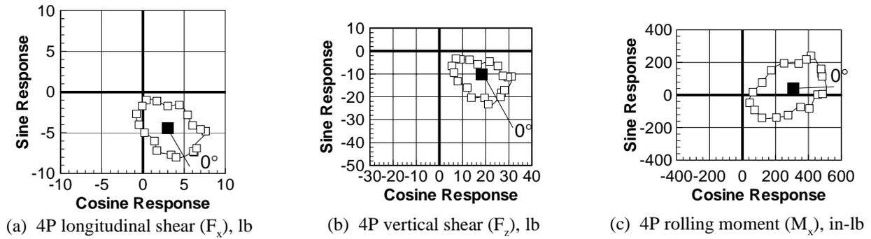
Figure 16. Response maps for  $\mu = 0.140$ ,  $C_L = 0.0066$ ,  $\alpha_s = -1.0^\circ$ , and 3P, 1000 V IBC actuation.
