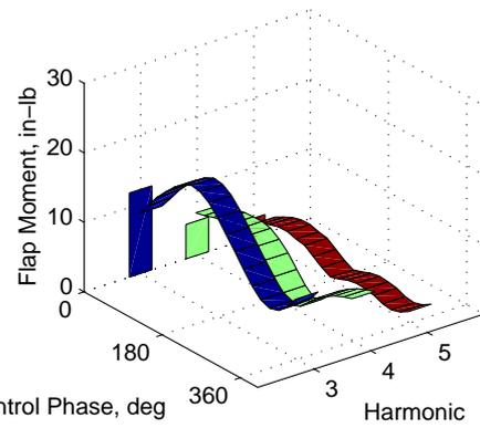
Figure 5. Sample ribbon plot. Blade flapwise bending moment (0.29R) for 3P IBC control.  $\mu = 0.140$ ,  $C_L = 0.0066$ ,  $\alpha_s = -1.0^\circ$ , and 1000 V actuation amplitude.
