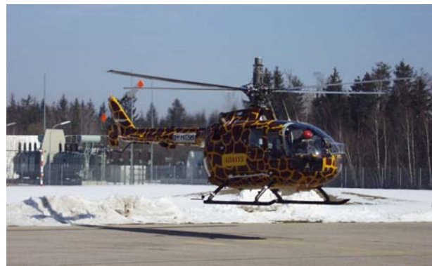
Figure 1: BO105 test bed for IBC by blade root actuation
