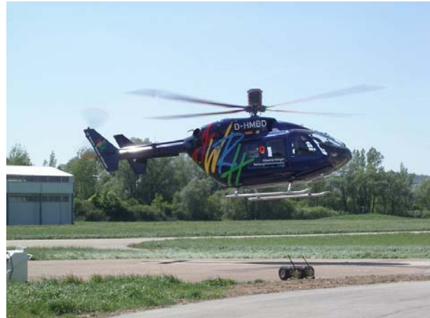
Figure 43: First flight of a helicopter with piezo actuated trailing edge flaps
