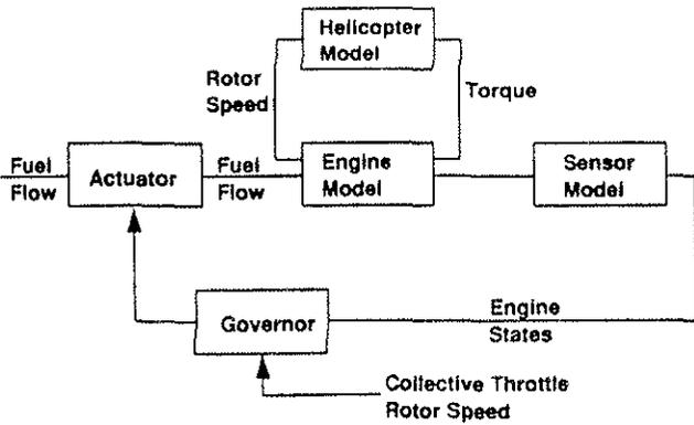
Fig. 8 Block diagram for the engine simulation model
