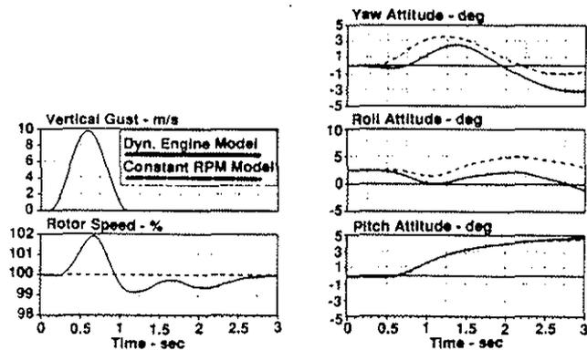
Fig.7 Calculated time histories due to vertical gust influence of rotor speed DOF
