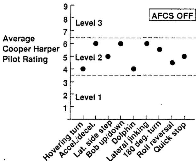
Fig. 18 Pilot ratings for some mission task elements - simulation tests
