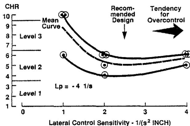
Fig. 22 CHR for a lateral unmask and remask task
