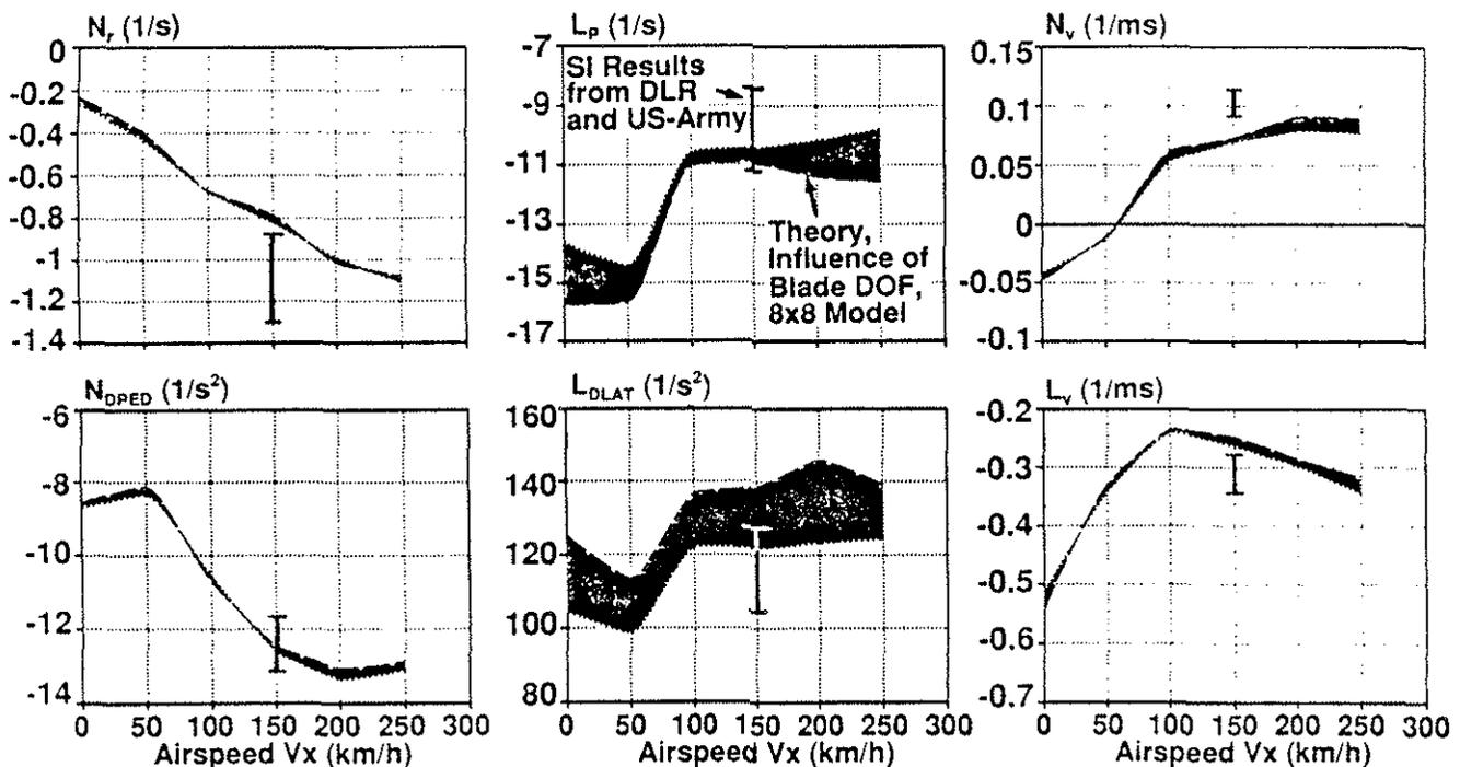
Fig. 12 Lateral derivatives for BO 105 system identification vs theory
