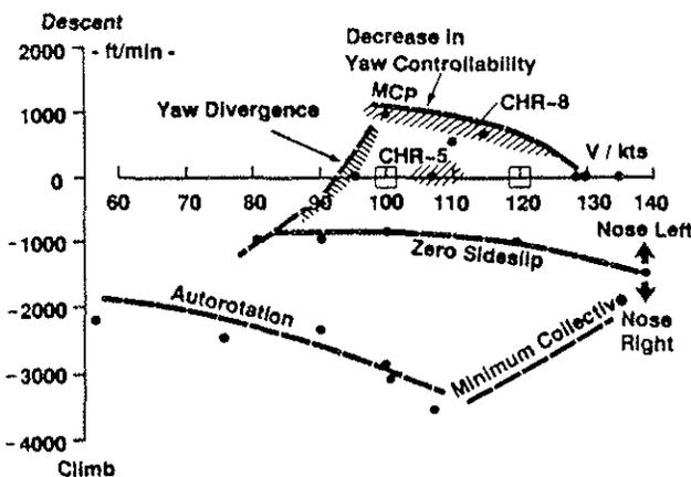
Fig. 26 Simulator study on flight envelope after tail rotor failure
