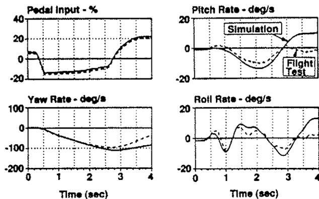
Fig. 15 Validation of a hover turn manoeuvre
