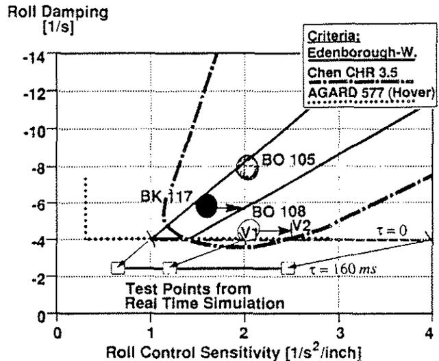
Fig. 23 Controllability - roll response
