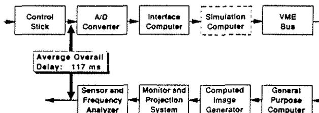
Fig. 11 Analysis of the simulator latency
