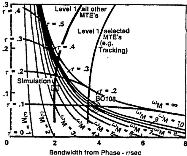
Fig. 25 Correlation of bandwidth low order equivalent system
