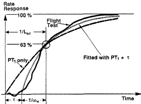
$L_{p,f}$  : Roll damping fitted to flight test without time delay
