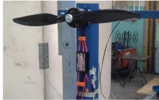
Fig. 1. The propeller (R380 30x5.5) with Turnigy RotoMax 150cc electric motor
