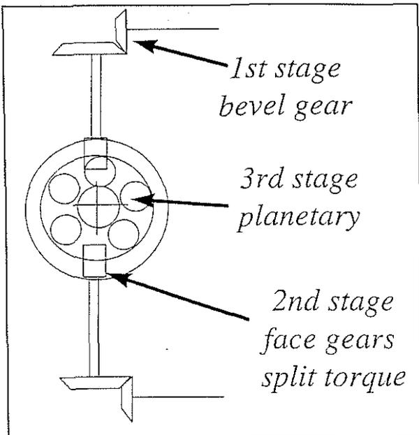
Face Gear Architecture - Two Stage Approach (Figure 2)
