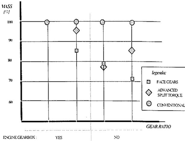
For relatively low Drive Train gear ratios, the Face Gear architectures do not offer significant advantages since part of the speed reduction is achieved within the engine and the rest of speed reduction is well feasible by conventional approaches with comparable mass figures (bevel and planetary gears).
