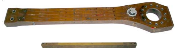
Fig. 1. Elastic hub of “Ansat” helicopter
