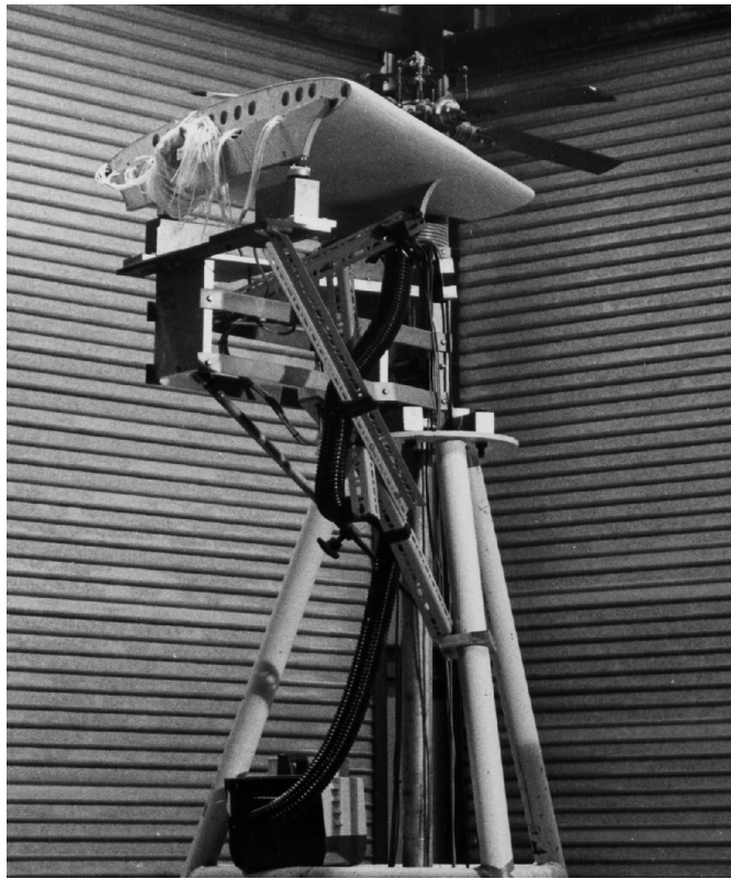
Figure 18. Experimental Set-up for Tail Rotor Fin-Blockage Tests (WHL 1980).
