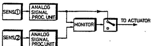
ANALOG DUAL CHANNEL SYSTEM WITH CROSS CHANNEL MONITORING
