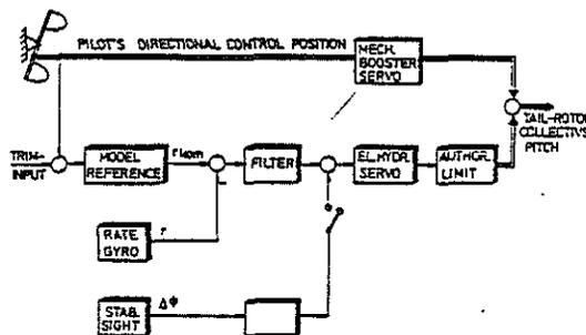
Fig.1: Typical Helicopter CSAS
