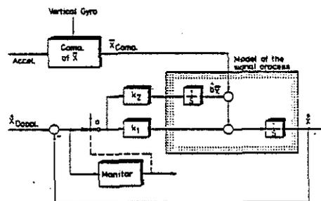
Fig. 9: MONITORING CONCEPT USING A
