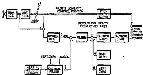
Fig.2: Advanced Helicopter (Hover) Control System - Pitch Axis
