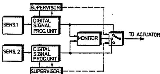
DIGITAL DUAL CHANNEL SYSTEM WITH SELF-AND CROSS CHANNEL MONITORING
