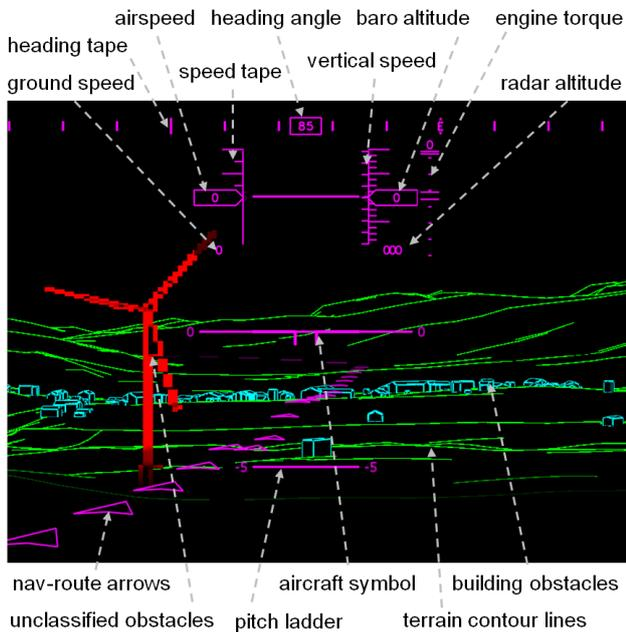
**Fig. 5: Example of a color-coded 2D and 3D-conformal display combination with different frames of reference**
