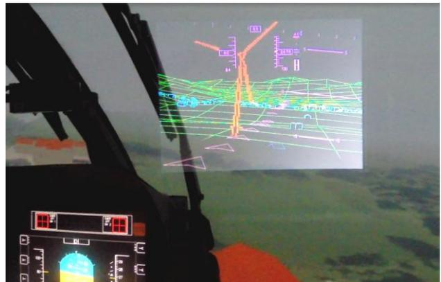
Fig. 1: Visual augmentation of the outside cues in ROSIE looking through the HMD (visual range 400 m)
