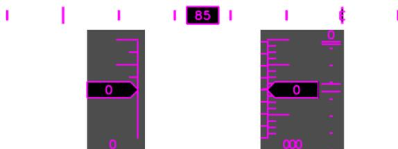
**Fig. 6: Background blending elements to ensure readability of the rotorcraft state parameters**
