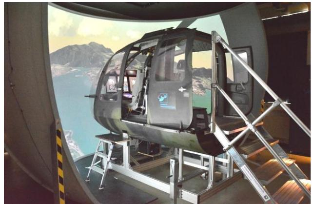
**Fig. 12: Rotorcraft Simulation Environment (ROSIE)**
