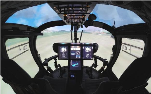
**Fig. 13: Cockpit view of ROSIE with four display configuration**
