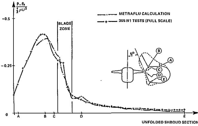
Fig.-11- Static pressure computation on the shroud
