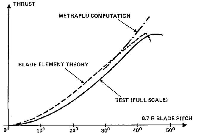
Fig.-13- Predicted and measured fenestron thrust versus pitch characteristic
