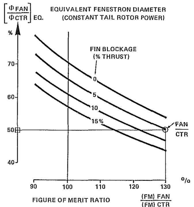
Fig.-24- Determination of fenestron / conventional tail rotor equivalent diameter at constant power
