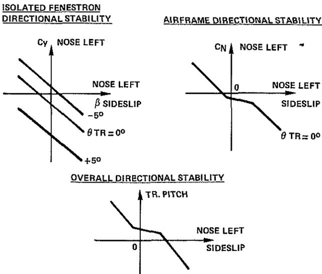
Fig.-4- Yaw stability in forward flight
