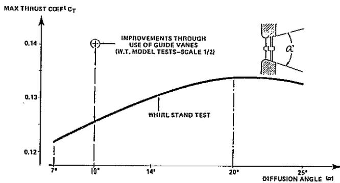
Fig.-17- Influence of diffuser angle and stator blades on fenestron performance
