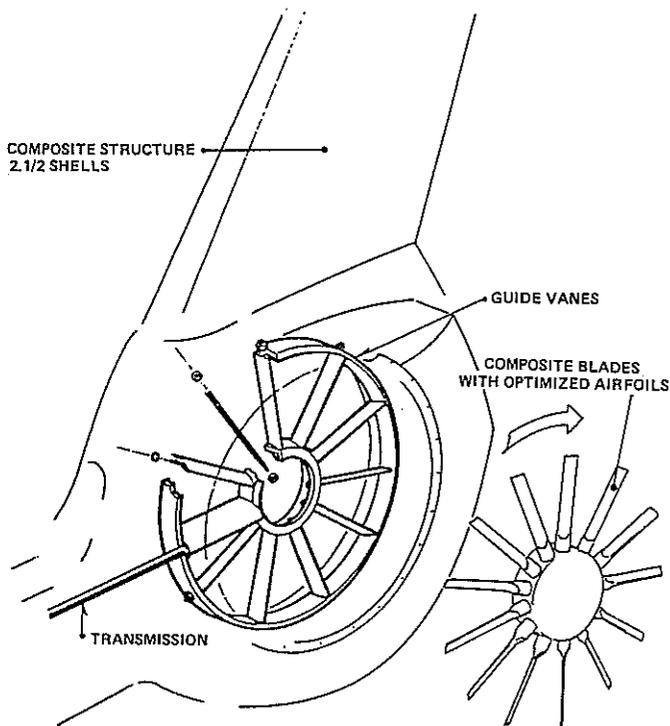
Fig.-2- Light helicopter composite fan in fin
