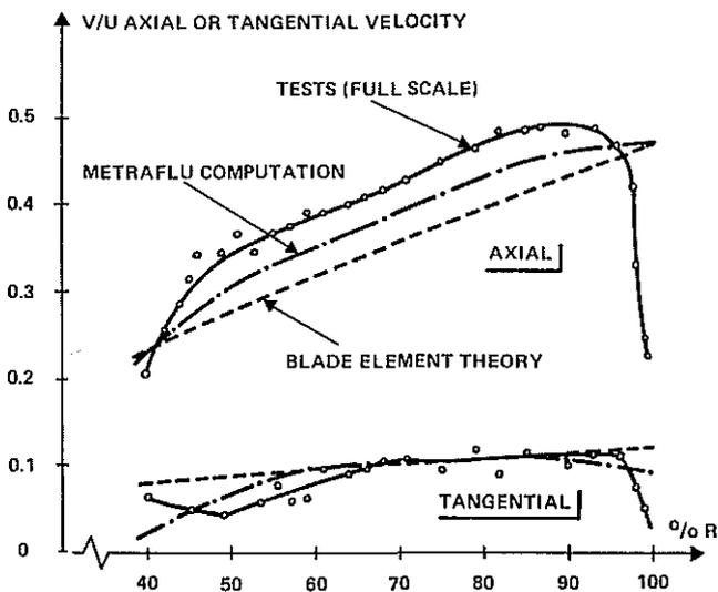
Fig.-12- Flow computation downstream the rotor blades
