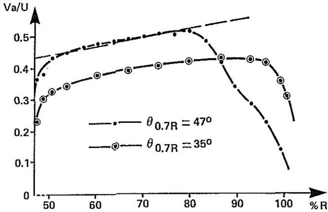
Fig.-8- Axial velocity distribution downstream the rotor blades
