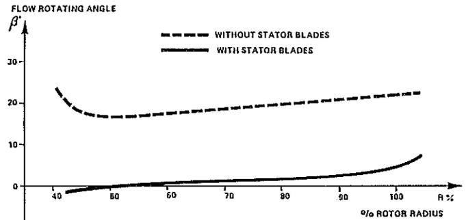
Fig.-19- Influence of stator blades on flow rotating angle at the diffuser exit
