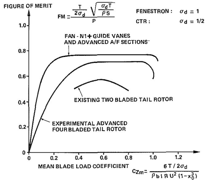
Fig.-23- Isolated tail rotor efficiency
