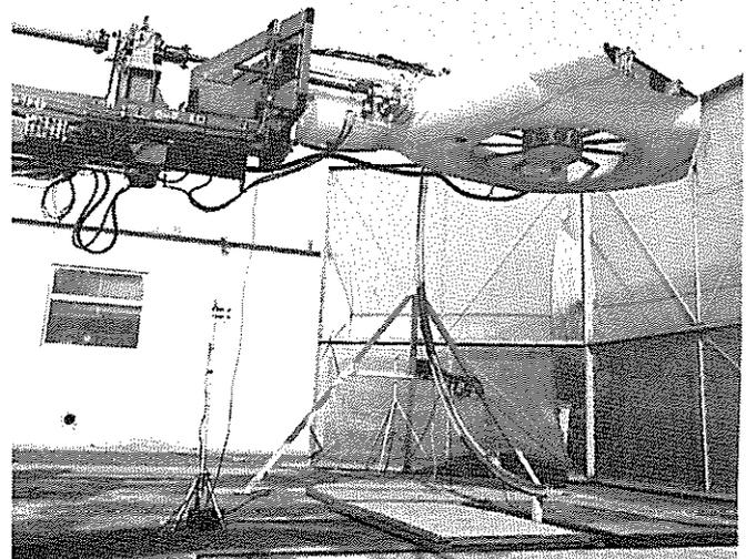
Fig.-20- Tail rotor research whirl test stand
