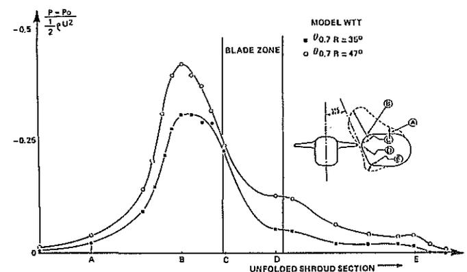
Fig.-7- Hover static pressure survey along the shroud
