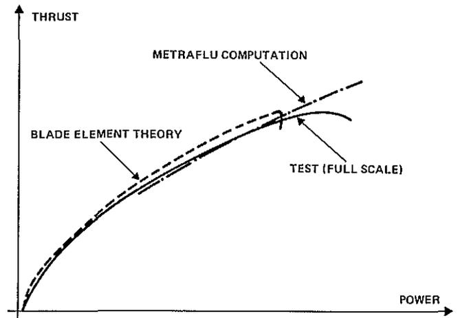
Fig.-14- Predicted and measured fenestron power versus thrust characteristic
