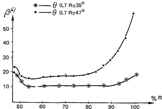
Fig.-9- Flow rotational angle downstream the rotor blades
