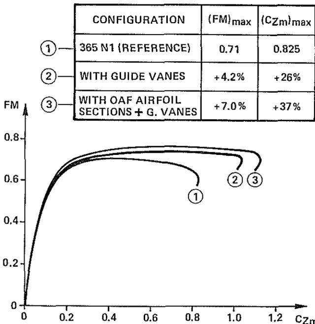
Fig.-22- Fenestron performance improvements (full scale ground tests)
