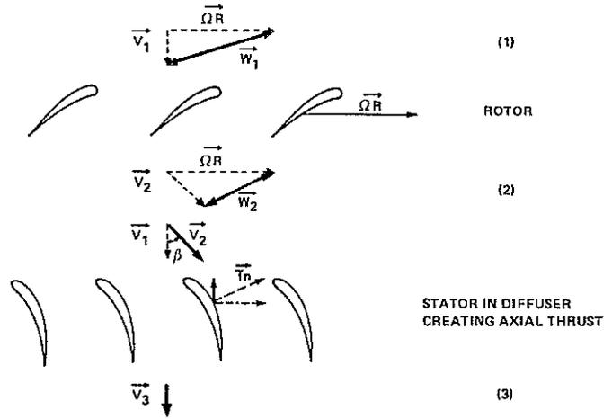
Fig.-18- Influence of stator blades on axial thrust
