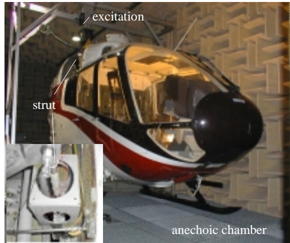
Figure 5 EC135 prototype fuselage / Smart strut (detail view)
