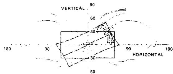
Fig. 3 Effect of display rotation on viewing area (from AH-1G - pilot's position).
