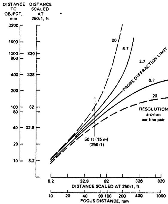
Fig. 11 Probe depth of field vs focus distance (from ref. 12).
