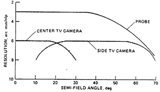
Fig. 10 Limiting resolutions vs field-of-view for probe and TV cameras (from ref. 12).
