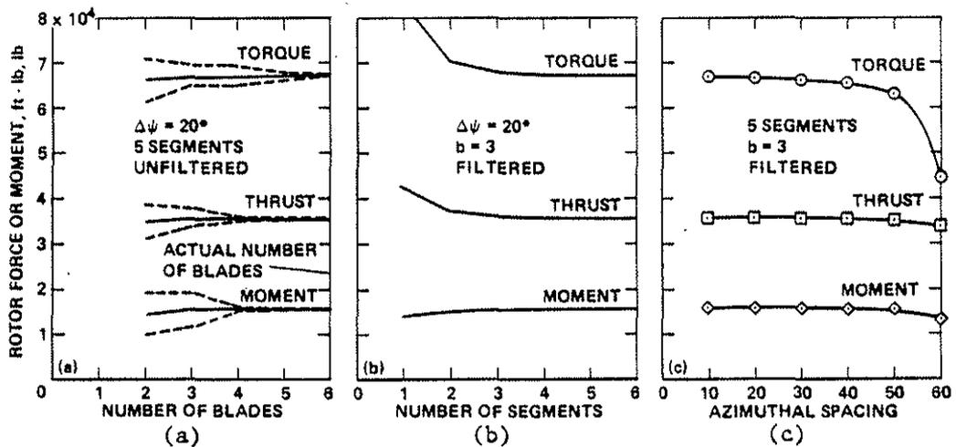
Fig. 14 Effect of blade truncation and azimuthal update on rotor force and moment output - 100 KTS (from ref. 25).
