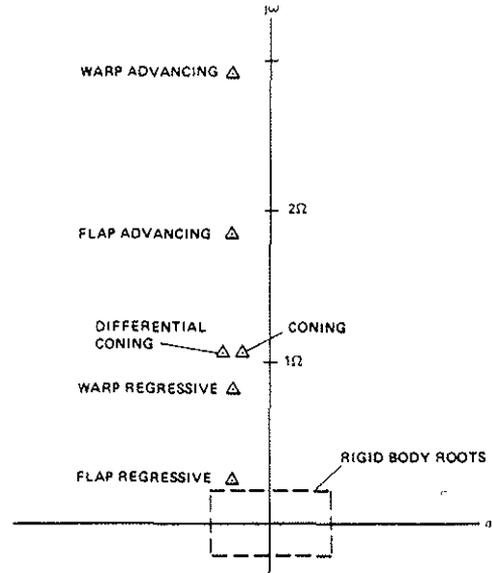
Fig. 13 Illustrative diagram plot showing typical characteristic root location for a six-bladed flapping rotor (from ref. 23).
