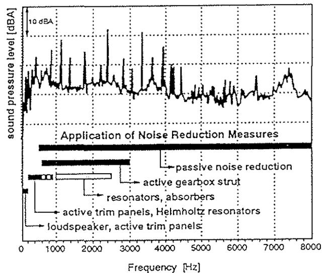
Figure 4: Typical Interior Noise Spectrum in an Untreated Small Size Helicopter and Noise Reduction Measures
