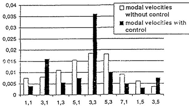
Figure 17: Modal Velocities on the Flat Panel with and without Active Control
