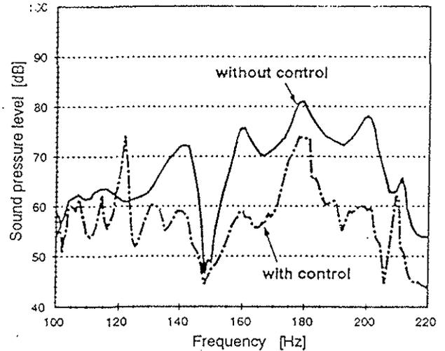
Figure 18: Sound Pressure Radiation of the Flat Panel with and without Active Control
