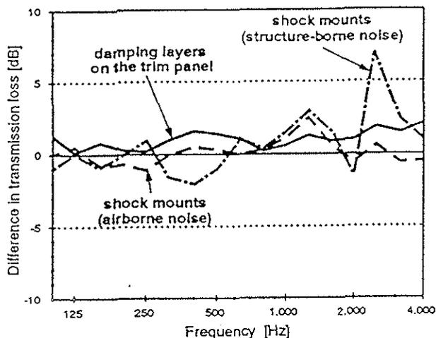
Figure 12: Effect of Shock Mounts and Damping Layers Applied to the Trim Panel
