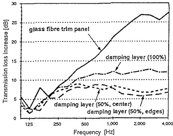
Figure 10: Increase in Transmission Loss of the Test Structure due to Various Damping Layer Configurations Compared to a GFRC Trim Panel (thickness 0.86 mm, weight 1.65 kg/m<sup>2</sup>)
