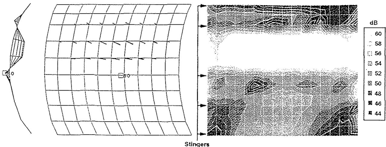
Figure 8: Sound Intensity Mapping of the 160 Hz-1/3-Octave Band and the Modal Analysis at 158 Hz
