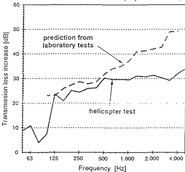
Figure 22: Measurement of the Interior Trim Package Inside the Helicopter Compared to Laboratory Measurements
