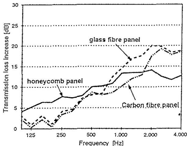
Figure 11: Increase in Global Transmission Loss due to Various Trim Panels Mounted on the Test Structure
