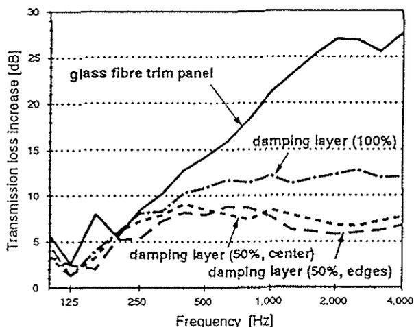
Figure 10: Increase in Transmission Loss of the Test Structure due to Various Damping Layer Configurations Compared to a GFRC Trim Panel (thickness 0.86 mm, weight  $1.65 \text{ kg/m}^2$ )
