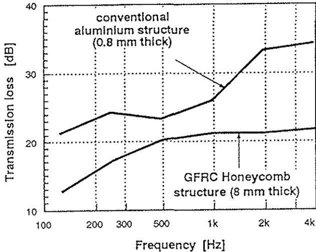
Figure 2: Transmission Loss of Pure Aluminium Structure and Honeycomb Structure (8 mm)
