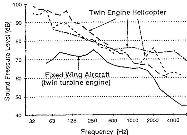
Figure 1: Interior Noise Levels of VIP-soundproofed Helicopters Compared to Fixed Wing Aircraft
