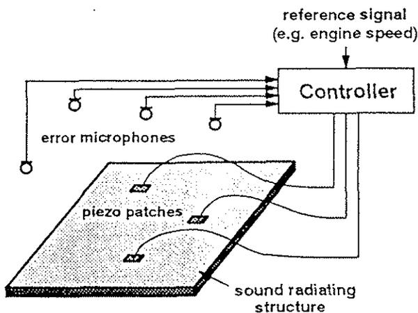
Figure 15: Scheme of an Active Panel Control System
