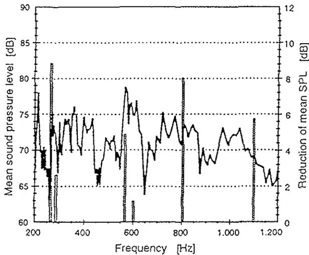
Figure 20: Mean Sound Pressure Level Radiated by the Test Structure and Noise Reduction by Active Control for Discrete Frequency Noise
