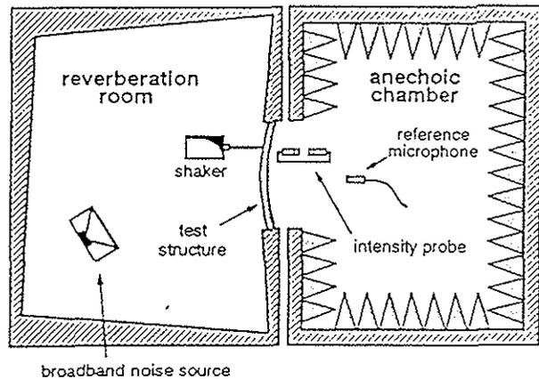
Figure 6: Measurement Arrangement
