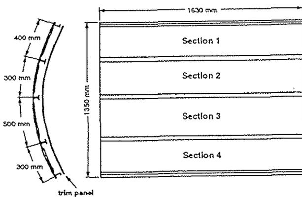
Figure 5: Helicopter Structure for Laboratory Tests
