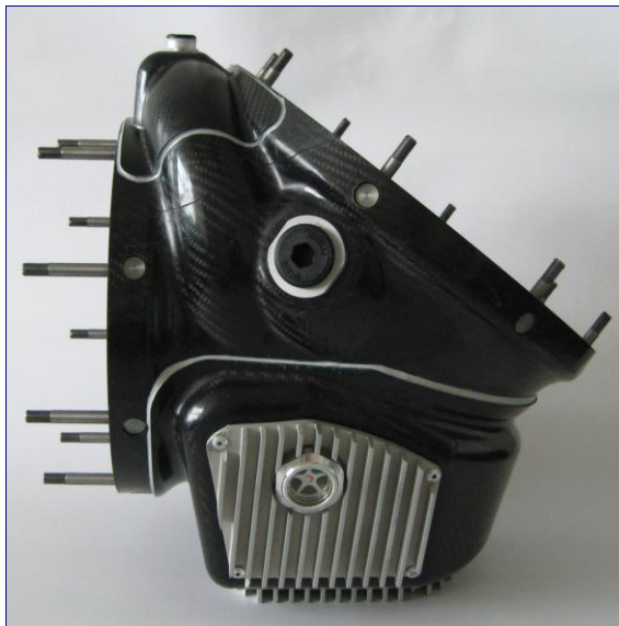
Figure 13: CFRP IGB housing including separate cooling areas and connecting elements
