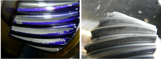
Figure 10: WC/C coated MGB bevel pinion at start (left) and at end (right) of testing
