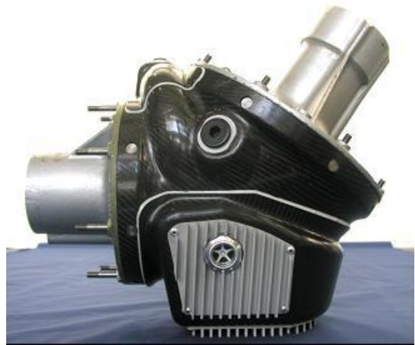
Figure 14: Assembled IGB using CFRP housing
