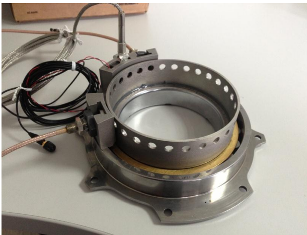
Figure 20: Main rotor mast bearing with integrated sensor technology [18] [19]
