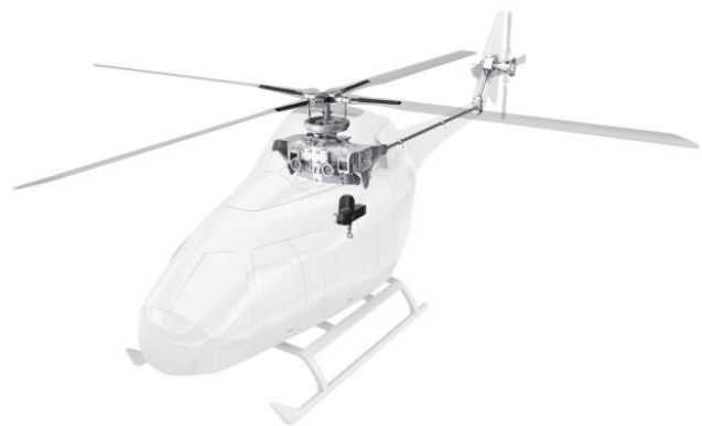
Figure 1: Typical drive-train layout of helicopter including MGB, IGB and TGB
