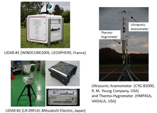
Fig. 8. Equipment used to measure helicopter wake.
