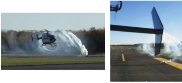
Fig. 17. Visualization of helicopter wake by smoke.
