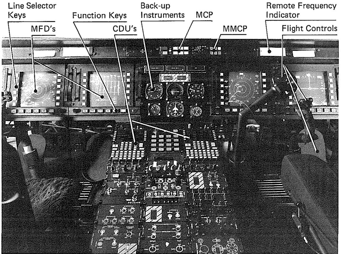
Figure 3: CMU Arrangement of Instruments and Panels
