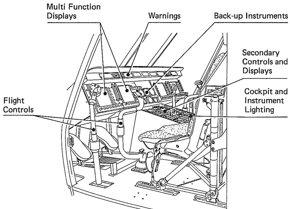
**Figure 2: CMU Man-Machine Interface**
