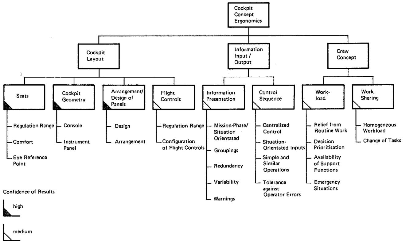
**Figure 1: Ergonomic Features of Cockpit Design**
