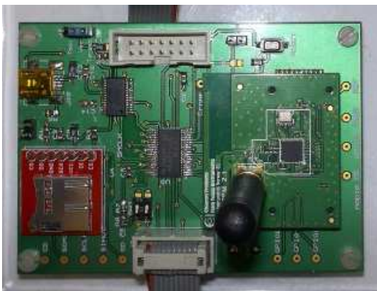
Figure 4. Prototype micro controller board with RF daughter board (on right hand side)
