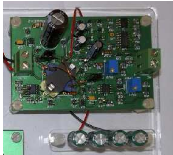
Figure 9. Photograph of the prototype power conditioning system .
