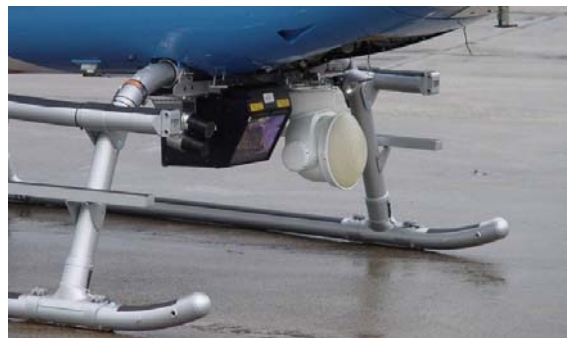
Figure 2: AI-130, HELLAS, FLIR and TV on DLR's research helicopter EC135
