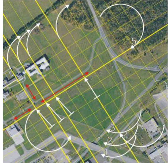
Figure 6: Obstacle detection trials (red – trucks movement, white – helicopter trajectory)
