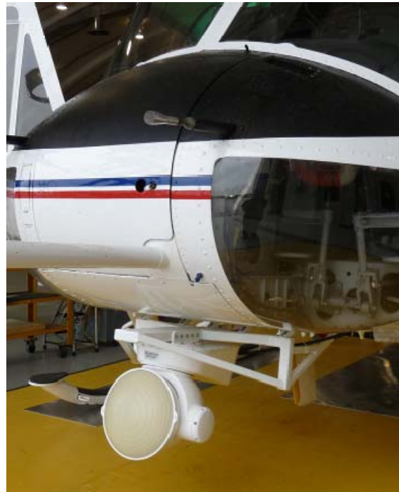
Figure 1: NRC's Bell 205 with the AI-130 radar
