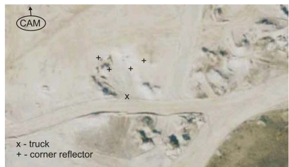
Figure 7: Aerial view of sandpit with truck, camera and corner reflector locations marked
