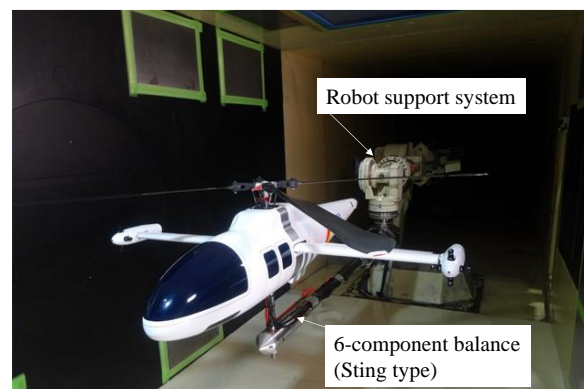
Figure 1. Experimental setup in test section at LWT2.
