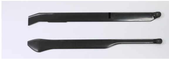
Figure 2. Blade model used in the wind tunnel test. (Upper: UH-60A blade, Lower: high- \mu BLN)
