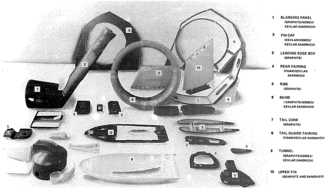
Fig. 13 EXPLODED VIEW OF DAUPHIN TAIL STRUCTURE
