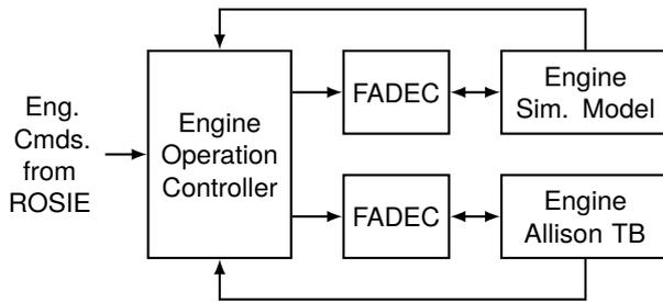
**Figure 5:** Integration of the EOC in the engine host
