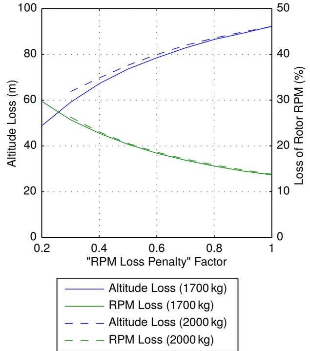
**Figure 9:** Loss of rotor speed and altitude
