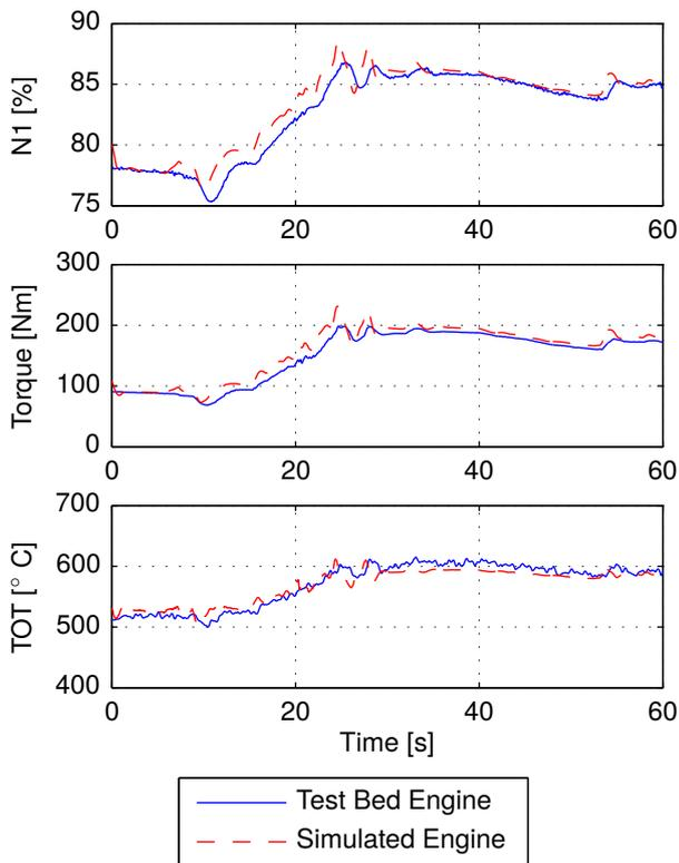
**Figure 6:** Comparison of engine measurements and simulation output in transient flight stages
