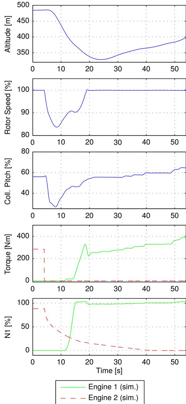
**Figure 7:** Simulated engine fail during manually piloted single engine operation
