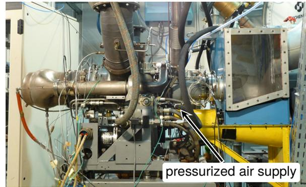
**Figure 4:** Allison 250-C20B at the engine test bed
