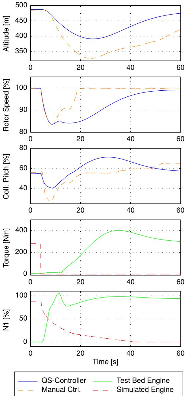
**Figure 10:** Engine-in-the-loop test: Power loss during ISEO with quick-start enabled flight control system and modified Allison 250-C20B
