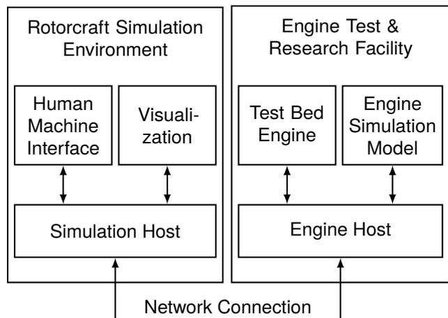
**Figure 2:** Scheme of simulator / test bed coupling
