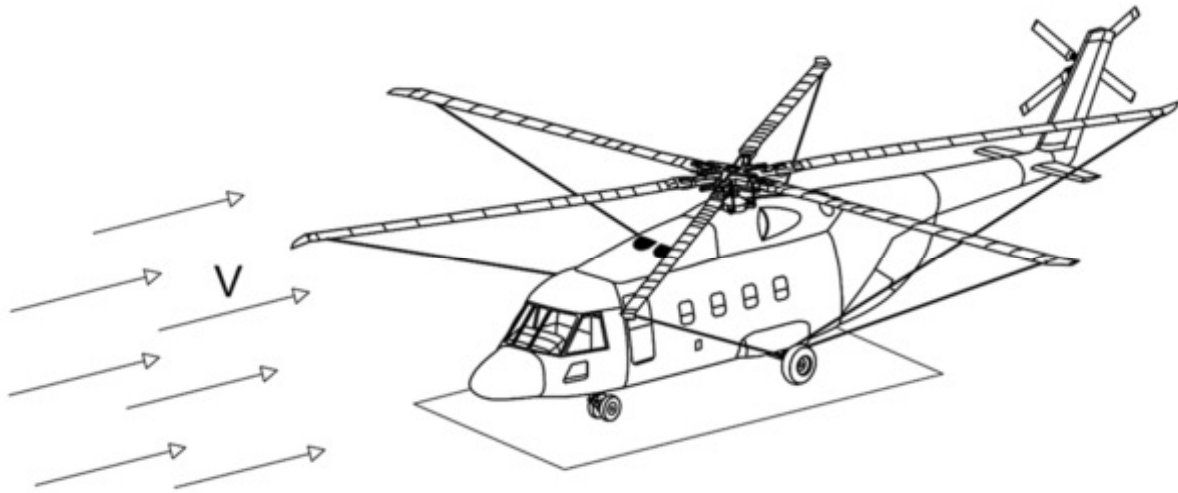
Figure 1: Moored main rotor blades under the influence of wind in the parking lot.
