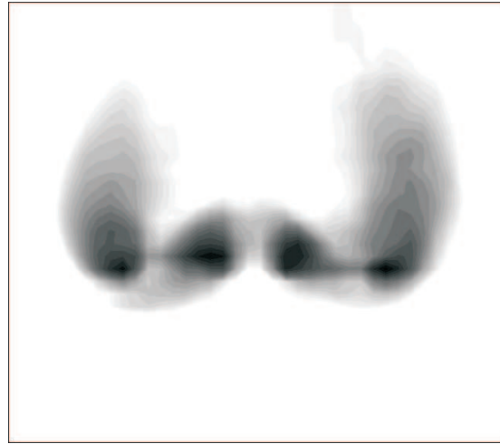
Figure 17: Averaged wake geometry at \bar{\mu}_z = 1.0 .
