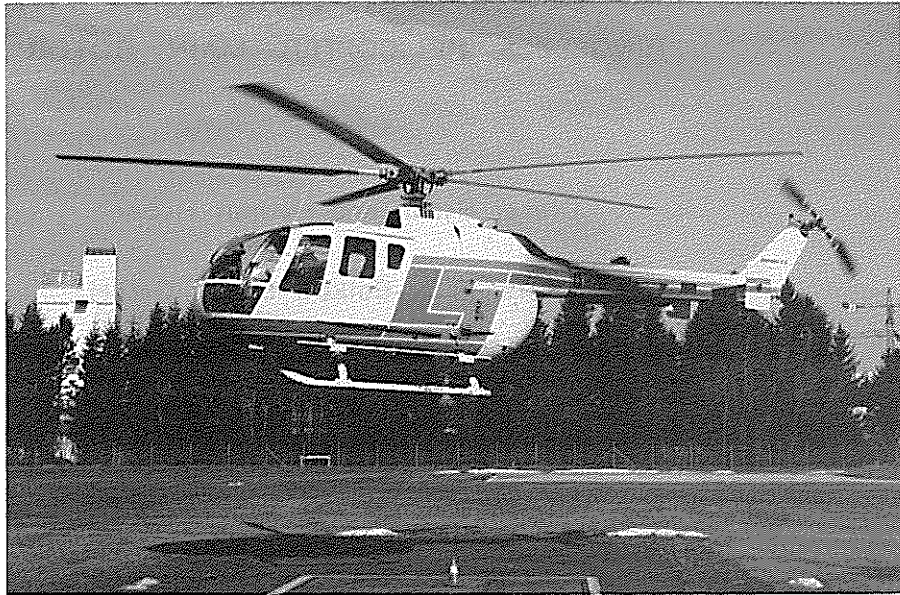
Fig. 1: 5-Bladed main rotor on BO 105 LS
