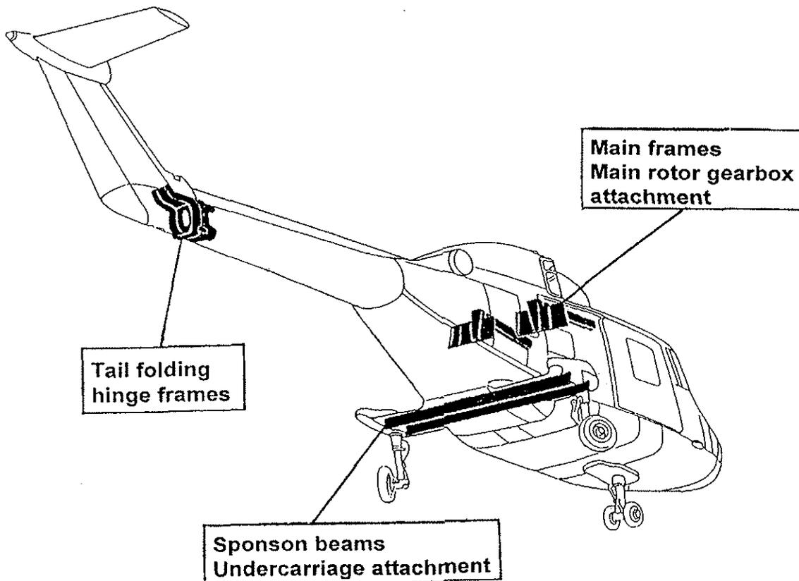
Figure 1: Fatigue sensitive and life limited area of Lynx airframe.
