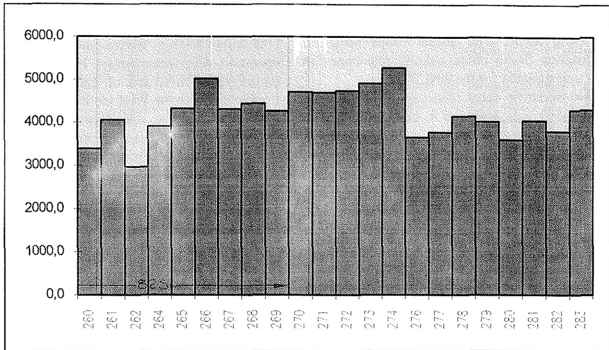
Figure 2: Distribution of consumed life over fleet: flying hours vs. aircraft registration number.
