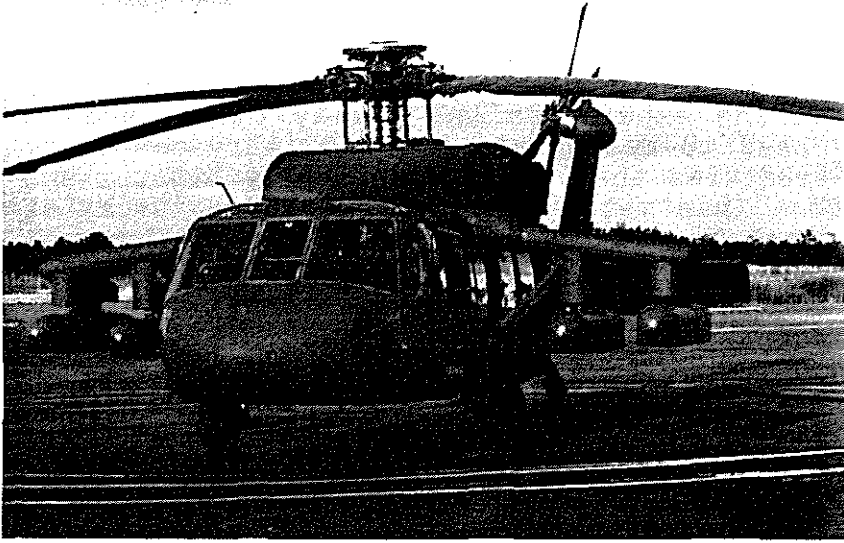
Figure 18. BLACK HAWK External Stores Support System
