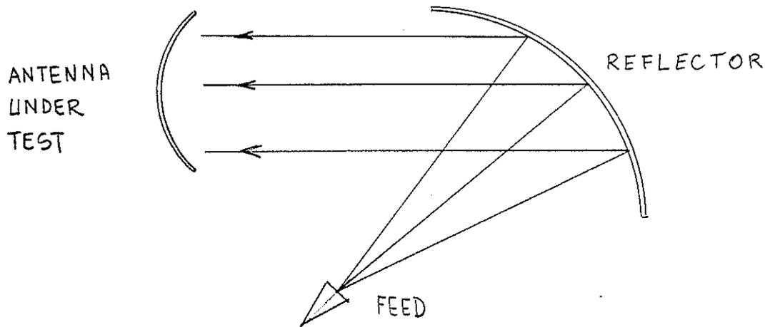
FIG. 6 SCHEMATIC REPRESENTATION OF A COMPACT RANGE EMPLOYING A REFLECTOR AND A FEED
