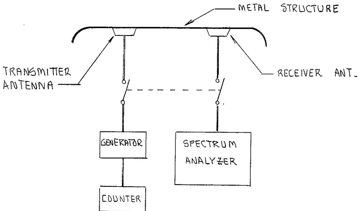
FIG. 9 ISOLATION MEASUREMENT TEST SET-UP
