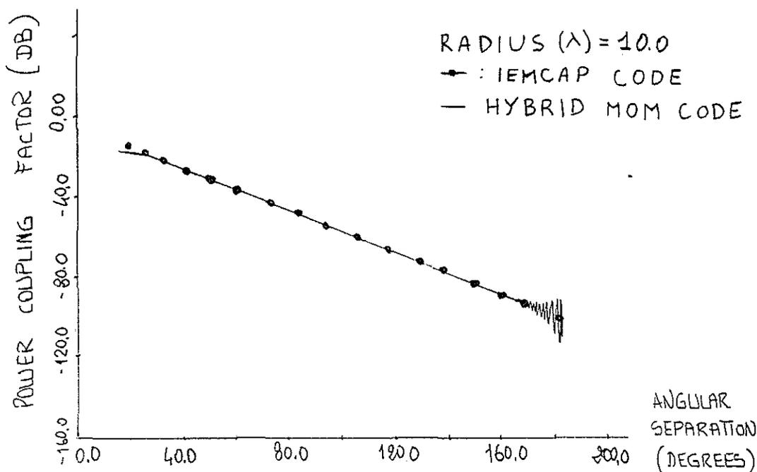
FIG. 8 POWER COUPLING FACTOR BETWEEN TWO  $1/4 \lambda$  MONOPOLES ON A CYLINDER OF RADIUS  $10 \lambda$
