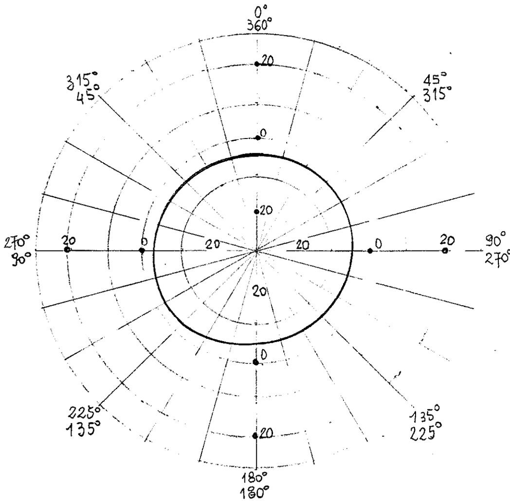
FIG. 3A. ANTENNA TYPE : HF LOOP      PLANE :  $\theta = 90^\circ$
