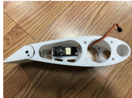
Figure 2: A wing section with deformable trailing-edge flap
