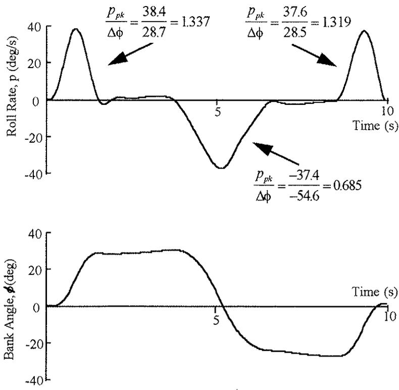
Figure 4: Calculation of roll quickness from inverse simulation of a rapid sidestep MTE.
