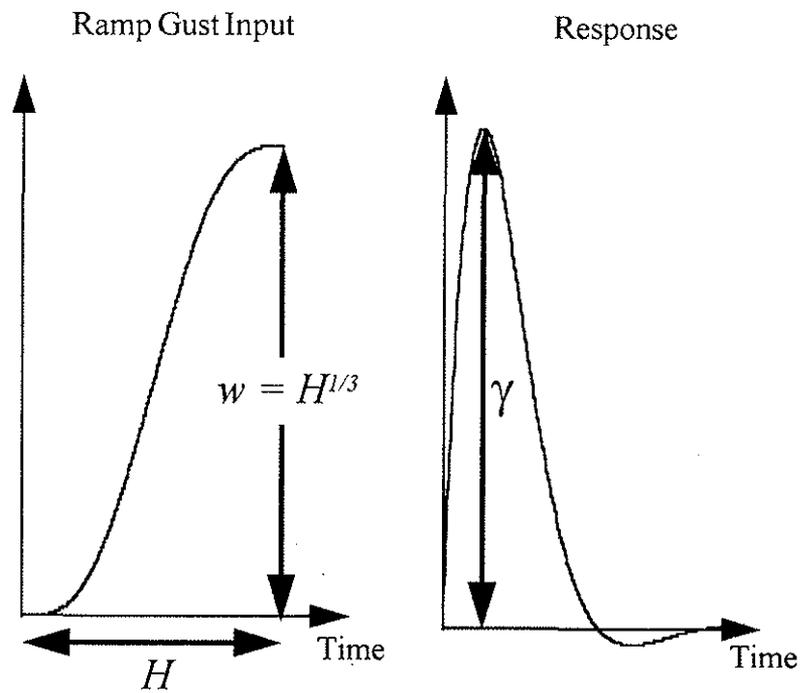
Figure 8: Ramp gust input with single peak response.
