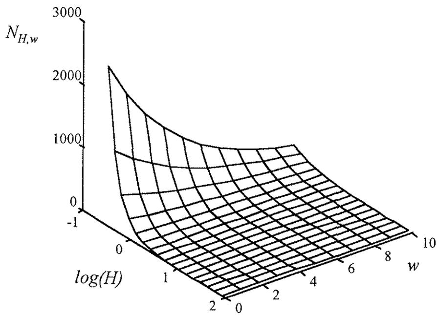
Figure 9: Number of gusts of ramp length  $H$  exceeding intensity  $w$  (SDG model).
