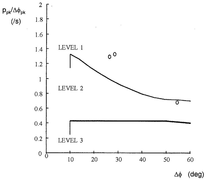
Figure 5: Roll quickness chart from inverse simulation of a rapid sidestep MTE.
