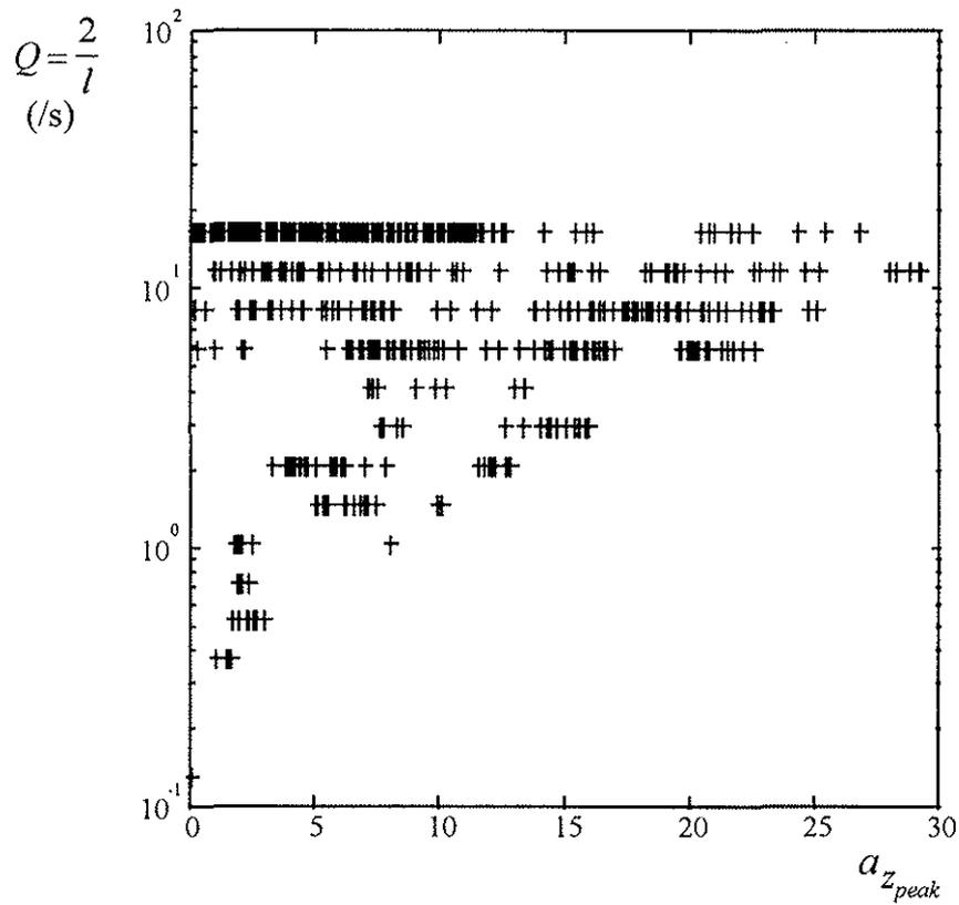
Figure 7: Quickness chart for response.
