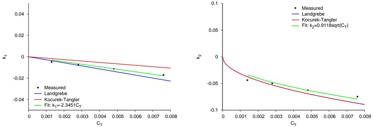
Figure 12: Axial convection rates for the untwisted blades
