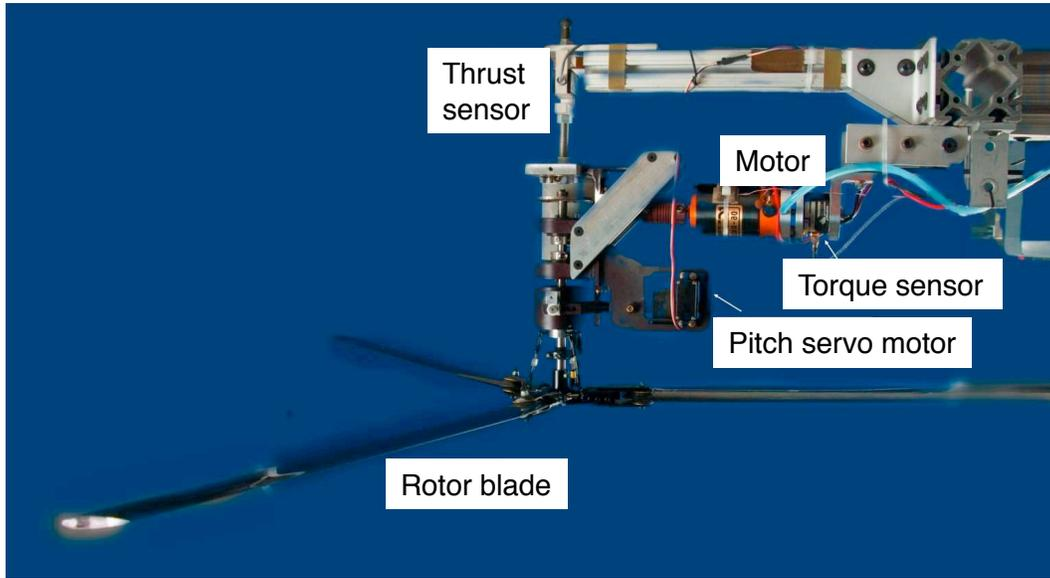
Figure 1: Close up view of the three-bladed rotor system.
