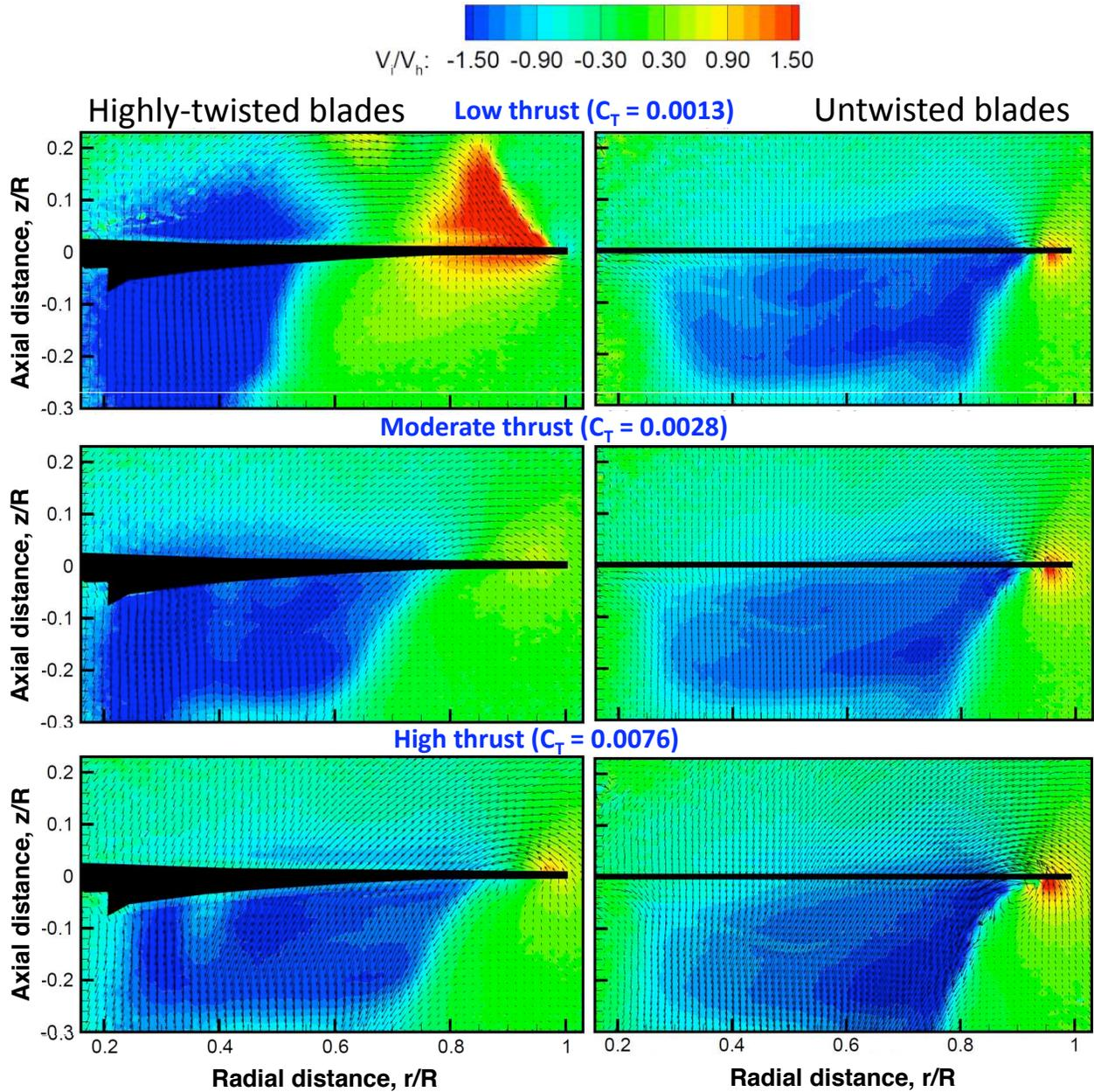
Figure 7: Time-averaged flowfield at higher thrust conditions
