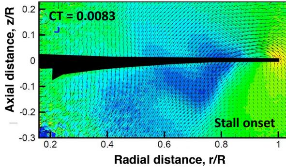
Figure 8: Time-averaged flowfield at stall for highly-twisted blade
