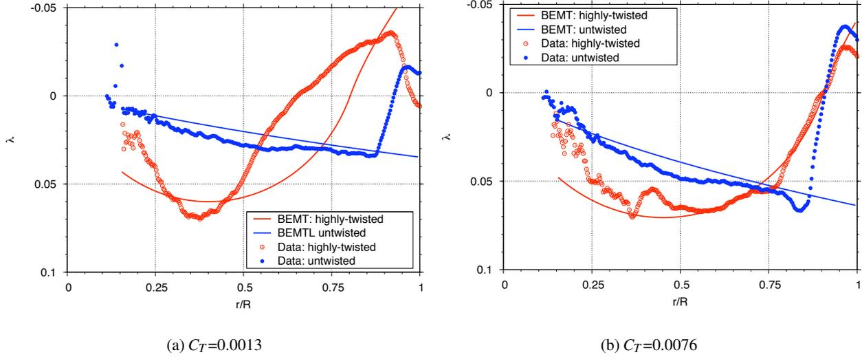
Figure 5: Averaged inflow at the rotor disk plane
