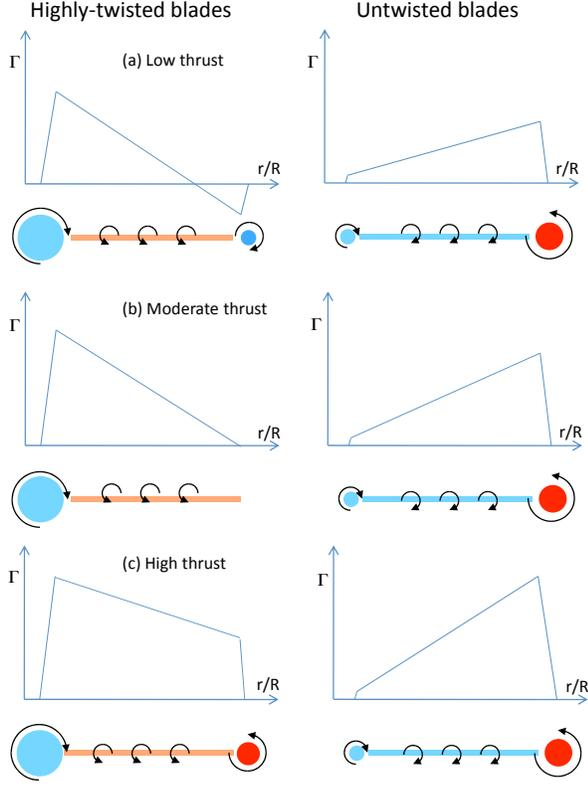
Figure 10: Schematic showing blade bound circulation and the resulting wake structure at different thrust conditions; (a)  $C_T=0.0013$ , (b)  $C_T=0.0028$ , and (c)  $C_T=0.0076$ .
