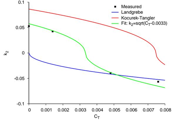
Figure 13: Axial convection rates for the highly-twisted blades
