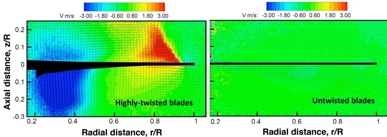
Figure 6: Time-averaged flowfield at zero thrust
