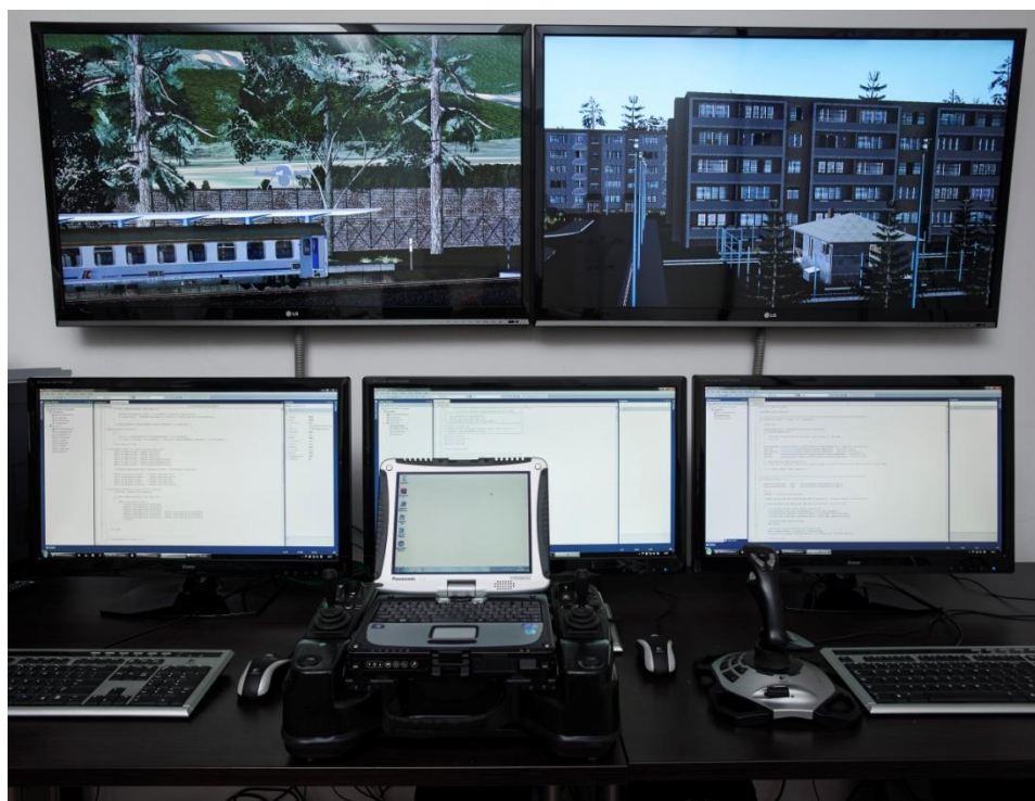
Fig. 1 The general view of the quadrotor training simulator
