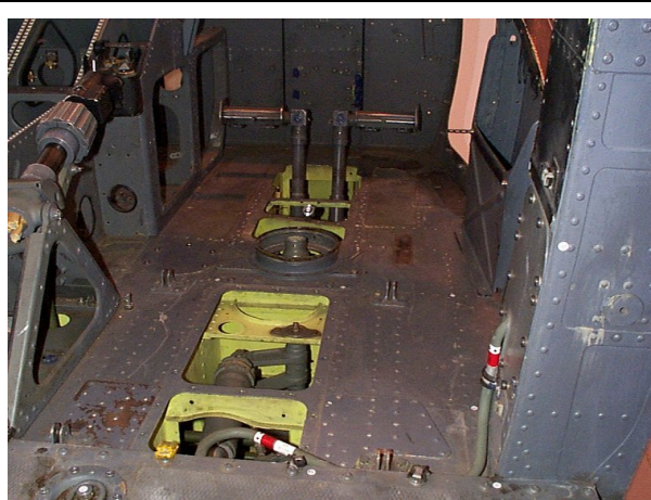
Figure 2: Control rods in cabin
